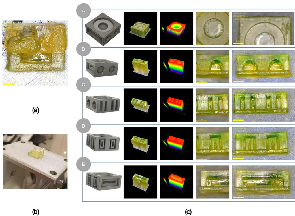
**Fig. 9** Photographs of prints obtained from a photo-cured resin: ANT-SCH<sub>3</sub>, IOD (0.1/1 w/w), 3% MDEA, CADE/TMPTA/M100 (2/2/1). (a) First attempt, (b) second attempt, (c) third attempt.
