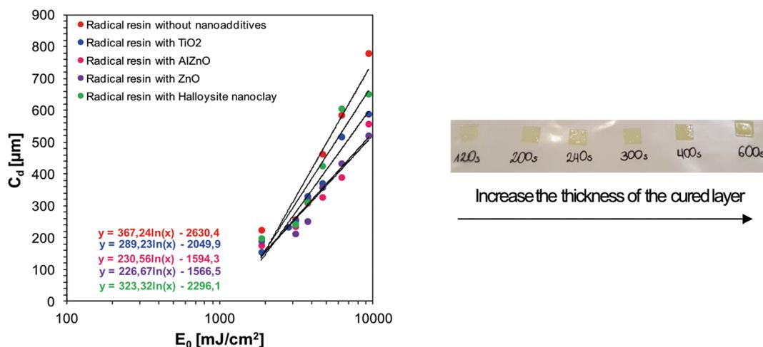
**Fig. 5** Determination of optimal printing parameters for a photo-curable resin: ANT-CH<sub>3</sub> + IOD (0.1/1 w/w) + 3% MDEA + HEMA/BEDA (3/7) without nano additives and with TiO<sub>2</sub>, AlZnO, ZnO and halloysite nanoclay; slices printed from ANT-CH<sub>3</sub> + IOD composition (0.1/1 w/w) + 3% MDEA + HEMA/BEDA (3/7) for Jacob's test.
