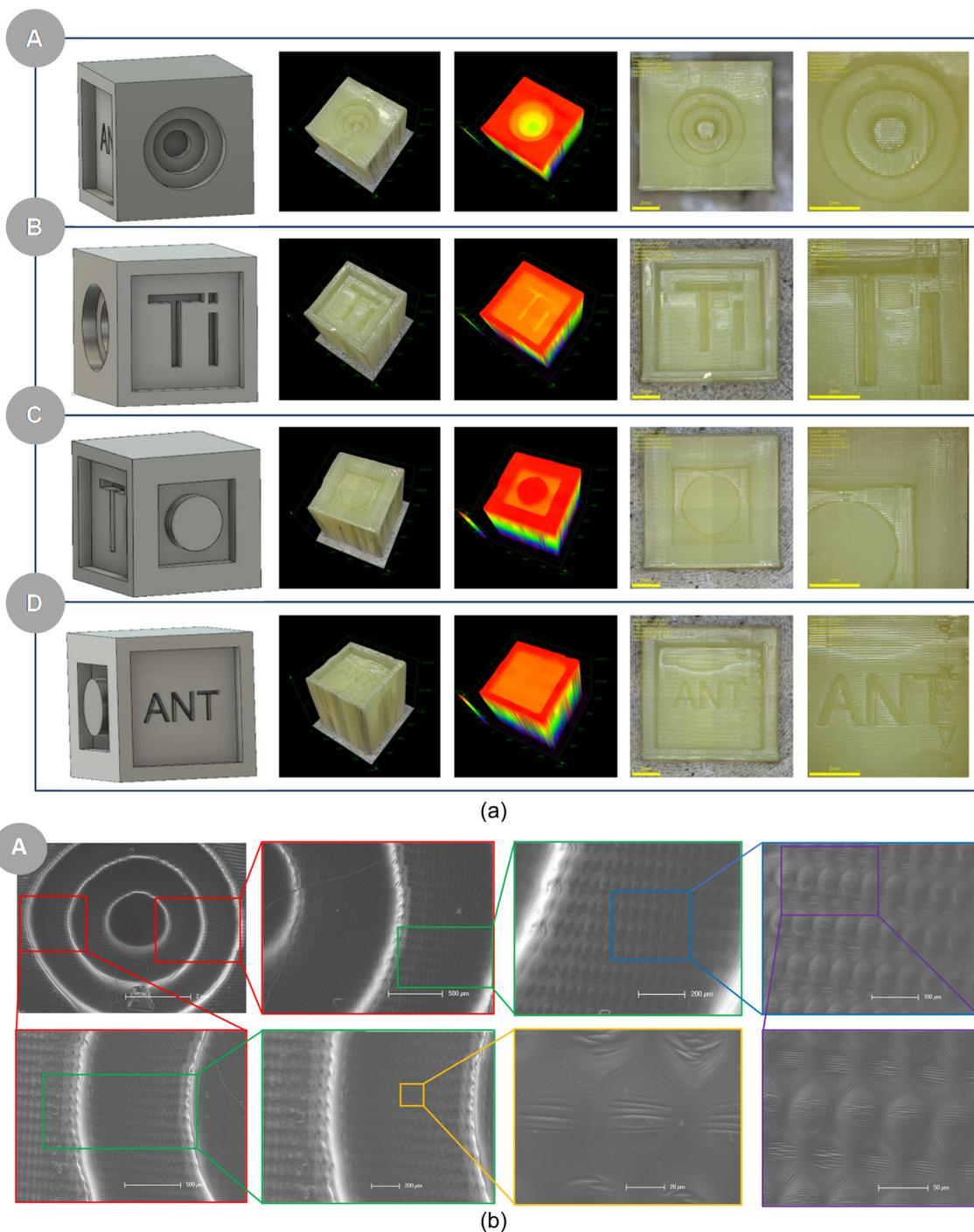
**Fig. 8** Photographs of a printout obtained from a photo-cured resin: ANT-CH<sub>3</sub>, IOD (0.1/1 w/w), 3% MDEA, HEMA/BEDA (3/7), 0.1% TiO<sub>2</sub> (A–D individual faces of a cube with different letters): (a) under an optical microscope, (b) under a scanning electron microscope.
