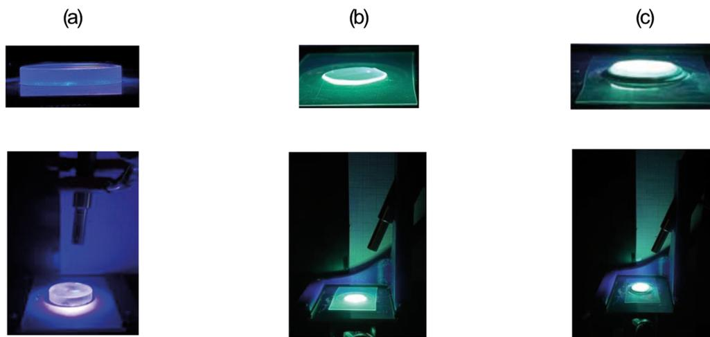
**Scheme 1** Images of the sample during measurements of photopolymerization kinetics under various conditions: (a) air conditions on a pastille (BaF<sub>2</sub> pastille, thickness 25  $\mu\text{m}$ , thin films); (b) laminated conditions (between PP films, thickness 25  $\mu\text{m}$ , thin films); (c) anaerobic conditions on rings ( $\varnothing = 9.80$  mm, thickness 1.16 mm, thick layers).
