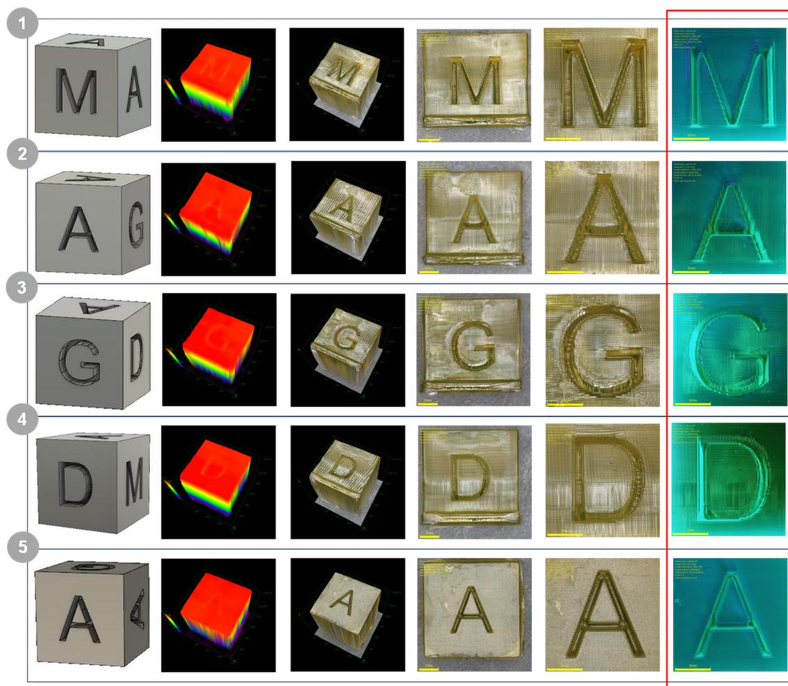
Fig. 7 Photographs of a printout obtained from a photo-cured resin: ANT-CH<sub>3</sub>, IOD (0.1/1 w/w), 3% MDEA, HEMA/BEDA (3/7) (1–5 individual faces of a cube with different letters); last column – photographs were taken under the UV flashlight.
