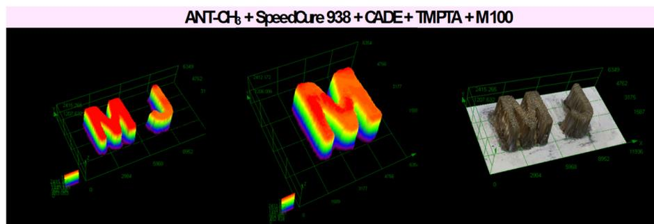
Fig. 6 Photographs of a 3D printout obtained from a hybrid composition based on ANT-CH<sub>3</sub> compound.
