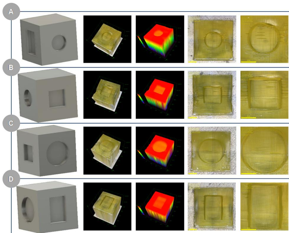
**Fig. 10** Photographs of a printout obtained from a photo-cured resin: ANT-SCH<sub>3</sub>, IOD (0.1/1 w/w), CADE/TMPTA/M100 (2/2/1) (A–D individual faces of a cube).
