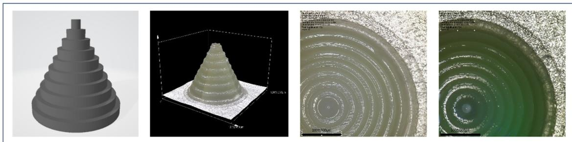
Fig. 11 Photographs of a printout obtained from a photo-cured resin: ANT-SCH<sub>3</sub>, IOD (0.1/1 w/w), CADE/TMPTA/M100 (2/2/1), 0.1% TiO<sub>2</sub>.
