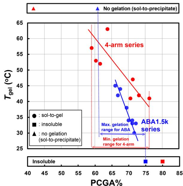
**Fig. 7** Comparison of the effect of PCGA% on gelation temperature ( $T_{\text{gel}}$ ) for linear ABA triblock and 4-arm branched PEG–PCGA copolymers. Circle: sol-to-gel transition, triangle: no gelation (sol to precipitation), and square: insoluble. Blue: ABA1.5k series (MW of PEG = 1540) and red: 4-arm PEG–PCGA series.
