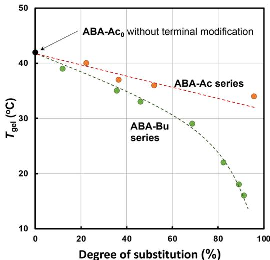
**Fig. 6** Effect of the degree of substitution (DS) (%) of terminal groups with acetyl or butyryl groups on the gelation temperature ( $T_{\text{gel}}$ ) of ABA triblock copolymers. ABA1.5k–3.1k–3.4 was used as the base polymer (ABA- $\text{Ac}_0$ ) for terminal modifications. Orange: acetyl, green: butyryl, and black: base polymer (ABA- $\text{Ac}_0$  = ABA1.5k–3.1k–3.4) without modification.
