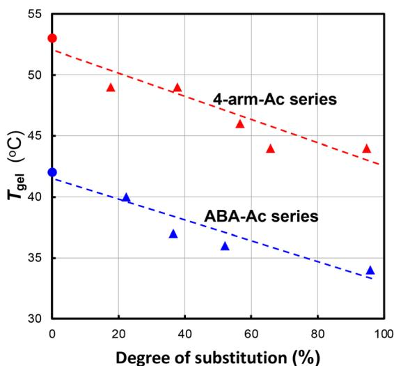
**Fig. 8** Effect of the degree of substitution (DS) (%) with acetyl groups on the gelation temperature ( $T_{\text{gel}}$ ) for linear ABA triblock (ABA-Ac series, the same data are shown in Fig. 5, blue) and 4-arm branched PEG-PCGA copolymers (4-arm-Ac series, red). For the 4-arm-Ac series, 4-arm5.0k–7.6k (4-arm-Ac<sub>0</sub>) was used as the base polymer for terminal modifications.
