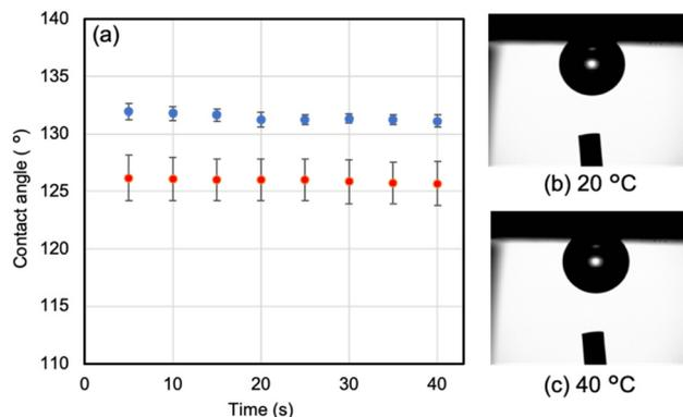
**Fig. 3** (a) Contact angles of air-in-water (captive bubble) for the P(DEGMA-*stat*-TEGMA)/PMMA heteroarm star-shaped polymer-coated surface at 20 and 40 °C. Photographic images of the captive bubbles at (b) 20 °C and (c) 40 °C.
