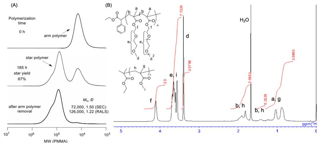
**Fig. 2** (A) SEC curves of P(DEGMA-*stat*-TEGMA)/PMMA (arm polymer) and the obtained heteroarm star-shaped polymer before and after arm polymer removal. (B)  $^1\text{H}$  NMR spectrum of the obtained heteroarm star-shaped polymer.
