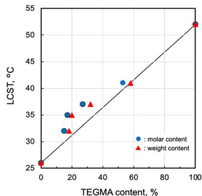
Fig. 1 Dependence of LCST on TEGMA content for P(DEGMA-*stat*-TEGMA). Circle: molar content; triangle: weight content.
