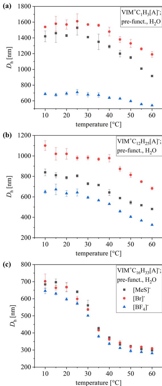
**Fig. 3** Hydrodynamic diameter ( $D_h$ ) as a function of alkyl chain length, counterion and temperature of pre-functionalized microgels. Temperature-dependent  $D_h$  of (a)  $\text{VIM}^+\text{C}_1\text{H}_3[\text{A}]^-$  microgels, (b)  $\text{VIM}^+\text{C}_{12}\text{H}_{25}[\text{A}]^-$  microgels, and (c)  $\text{VIM}^+\text{C}_{16}\text{H}_{33}[\text{A}]^-$  microgels with different counter anions.
