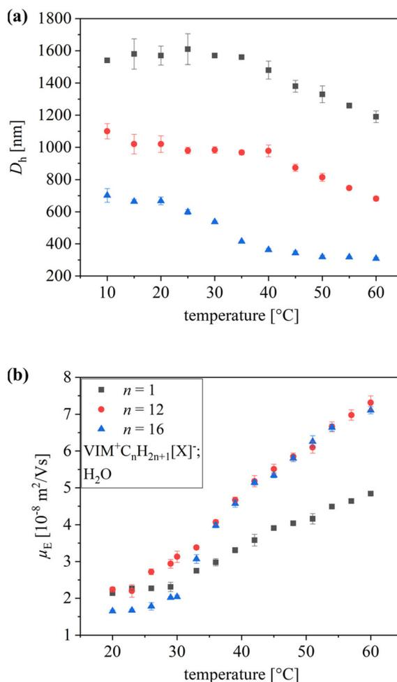
**Fig. 1** (a) Hydrodynamic diameter ( $D_h$ ), and (b) electrophoretic mobility ( $\mu_E$ ) of poly(VCL-co- $\text{VIM}^+\text{C}_n\text{H}_{2n+1}[\text{X}]^-$ ) microgels as a function of alkyl chain length, and temperature ( $n = 1$ , black squares;  $n = 12$ , red dots;  $n = 16$ , blue triangles).
