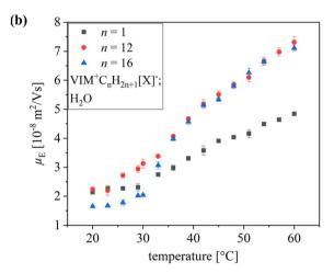
Fig. 1 (a) Hydrodynamic diameter  $(D_h)$ , and (b) electrophoretic mobility  $(\mu_{\rm E})$  of poly(VCL-co-VIM $^+$ C $_n$ H $_{2n+1}$ [X] $^-$ ) microgels as a function of alkyl chain length, and temperature (n = 1, black squares; n = 12, red dots; n = 116, blue triangles).
