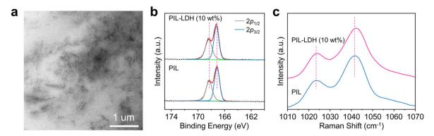
Fig. 2 (a) TEM image of the PIL-LDH composite containing 10 wt% LDH. (b) High-resolution S 2p XPS spectra and (c) Raman spectra of the PIL and PIL-LDH composite containing 10 wt% LDH.
