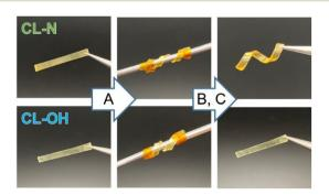
Fig. 4 Difference of reprocessability between CL-N and CL-OH during the process with A: fixing the sample with kapton tapes, B: heating in an oven (150  $^{\circ}$ C, 30 min), and C: cooling to 25  $^{\circ}$ C (room temperature).
