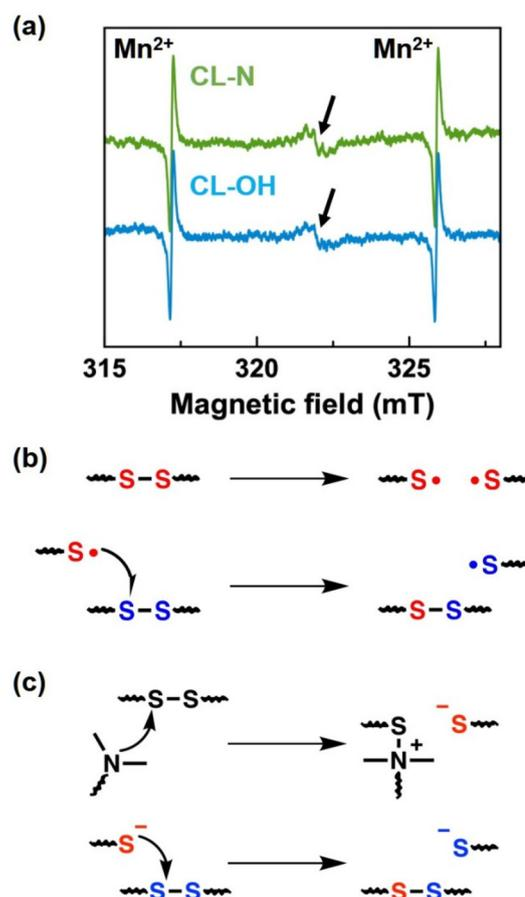
**Fig. 5** (a) ESR spectroscopy data for CL-N and CL-OH measured at  $160 \text{ }^\circ\text{C}$ . The arrows represent the signal from the sulfide radical, and the distinct outside signals were from  $\text{Mn}^{2+}$  used for the magnetic field calibration. (b) The bond exchange mechanism of the disulfide bond via a radical-mediated mechanism and (c) a thiolate anion-mediated mechanism in the presence of tertiary amines.
