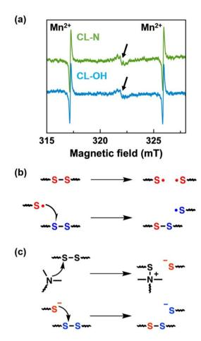
Fig. 5 (a) ESR spectroscopy data for CL-N and CL-OH measured at 160 °C. The arrows represent the signal from the sulfide radical, and the distinct outside signals were from  $\mathrm{Mn^{2+}}$  used for the magnetic field calibration. (b) The bond exchange mechanism of the disulfide bond via a radical-mediated mechanism and (c) a thiolate anion-mediated mechanism in the presence of tertiary amines.
