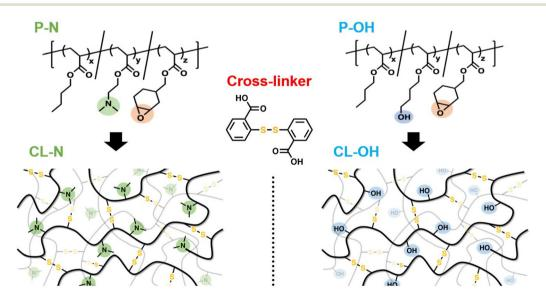
Fig. 1 Schematic diagrams of the precursor polymers and network designs for exploring the effects of internal tertiary amines on the disulfide bond exchange in the network.
