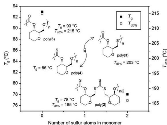
Fig. 5 Glass transition and degradation temperatures of poly(2–5) vs. the quantity of sulfur atoms in their monomers. Notable omissions include: poly(3) (no  $T_g$  detected) and poly(4) ( $T_{d5\%} = 136$  °C).
