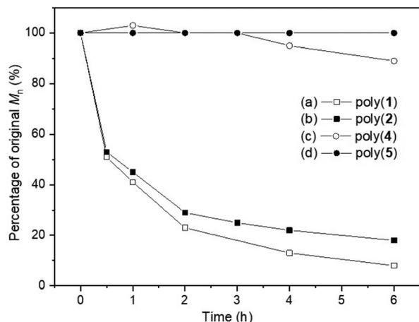
**Fig. 6** Plot of original  $M_n$  percentage vs. time, following the degradation of poly(1) ( $M_{n,SEC} = 10\,000\text{ g mol}^{-1}$ ,  $D_M = 1.77$ ),<sup>21</sup> poly(2) ( $M_{n,SEC} = 5500\text{ g mol}^{-1}$ ,  $D_M = 1.54$ ), poly(4) ( $M_{n,SEC} = 6300\text{ g mol}^{-1}$ ,  $D_M = 1.30$ ) and poly(5) ( $M_{n,SEC} = 4900\text{ g mol}^{-1}$ ,  $D_M = 1.16$ ) when exposed to UV light ( $\lambda = 365\text{ nm}$ ) for 6 hours, at room temperature, in THF solution.
