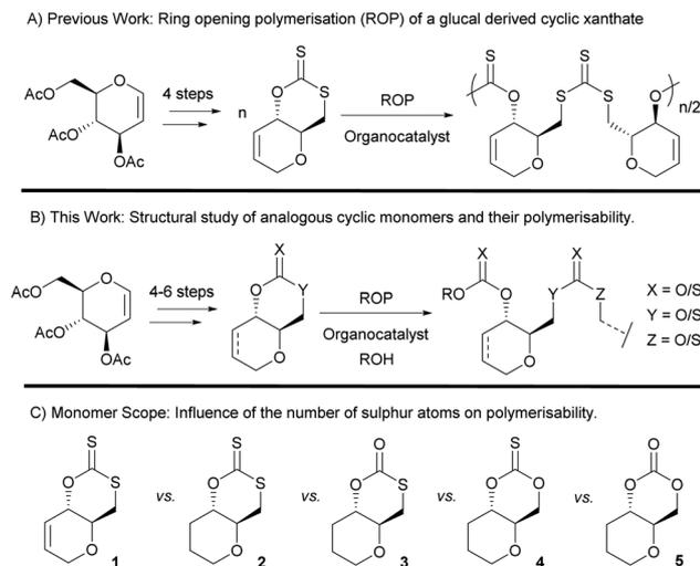
**Fig. 1** (A) Organocatalysed ring opening polymerisation of a cyclic xanthate; (B) organocatalysed ring opening polymerisation of novel cyclic monomers and investigation of polymerisability and the properties of resultant polymers; (C) concept of exploring quantity and arrangement of sulfur atoms within the carbonyl/thiocarbonyl linkage.
