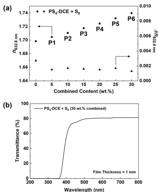
**Fig. 4** Relationship between the refractive indices at 632.8 nm ( $n_{632.8\text{nm}}$ ), birefringence ( $\Delta n_{632.8\text{nm}}$ ), and the composition of thermosets prepared from BEPS and equal amounts of PS<sub>4</sub>-DCE and S<sub>8</sub> (a) and (b) UV-Vis transmittance of a 1 mm-thick polymer film obtained from 15 wt% each of PS<sub>4</sub>-DCE and S<sub>8</sub> in BEPS.
