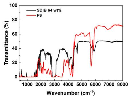
**Fig. 6** FT-IR transmittance spectra of 1 mm-thick samples of S-DIB prepared from inverse vulcanization and p(PS-BEPS) with 15 wt% each of PS<sub>4</sub>-DCE and S<sub>8</sub>.
