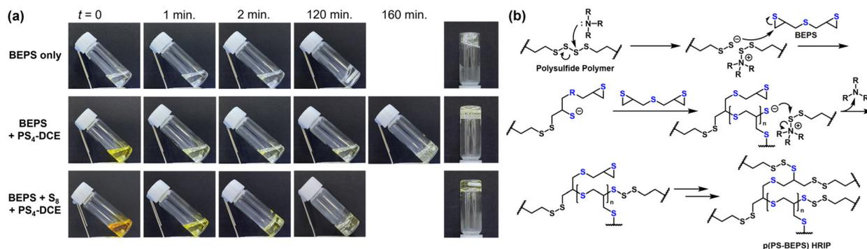
**Fig. 2** (a) Digital photographs of the amine-catalyzed polymerization of BEP, BEPS containing PS<sub>4</sub>-DCE (15 wt%), and BEPS containing 15 wt% each of PS<sub>4</sub>-DCE and elemental sulfur (S<sub>8</sub>) at 60 °C, with  $t = 0$  indicating the time at which the dicyclohexyl methyl amine catalyst was added, and (b) the proposed mechanism of the polymerization of BEPS and PS<sub>4</sub>-DCE giving a high refractive index thermoset.
