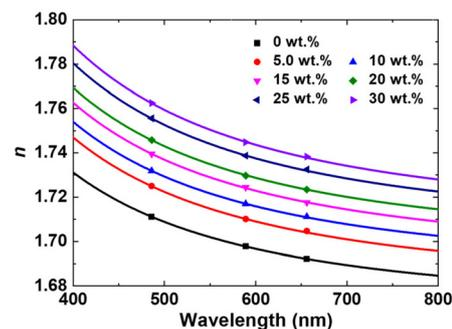
**Fig. 5** Wavelength-dependent refractive indices of BEPS copolymers prepared with various PS<sub>4</sub>-DCE/S<sub>8</sub> loadings.
