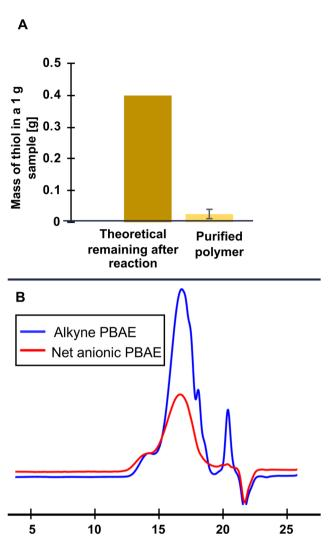
Fig. 2 Purification of net anionic PBAE by preparative SEC: (A) the reduction of thiol content averaged across all samples, measured by Ellman's assay, after preparative SEC purification, the error bar represents standard deviation (n = 7); and (B) differential refractive index analytical SEC chromatogram of the 100% HDDA alkyne functionalized PBAE and the same polymer after thiol—yne functionalization and preparative SEC under basic (pH = 9) conditions.
