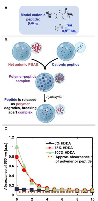
Fig. 5 Complexation of net anionic PBAEs with cationic species: (A) structure of model cationic peptide (GR)<sub>10</sub>; (B) scheme showing proposed complexation of (GR)<sub>10</sub> with net anionic PBAEs; (C) absorbance at 550 nm as a function of time of complexes of  $(GR)_{10}$  and net anionic PBAEs with 0, 75, or 100% HDDA-containing repeating units at a 1:1 charge ratio.
