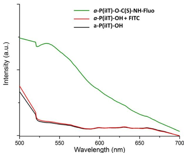
Fig. 6 Fluorescence emission studies for *a*-P(iIT)-OH (control, black line), *a*-P(iIT)-OH dipped in fluorescein solution (control, red line) and fluorescein-functionalized *a*-P(iIT)-O-C(S)-NH-Fluo (green line) thin films on SiO<sub>2</sub> in the solid state. All samples were excited at 495 nm and monitored for fluorescence emission between 500–700 nm.
