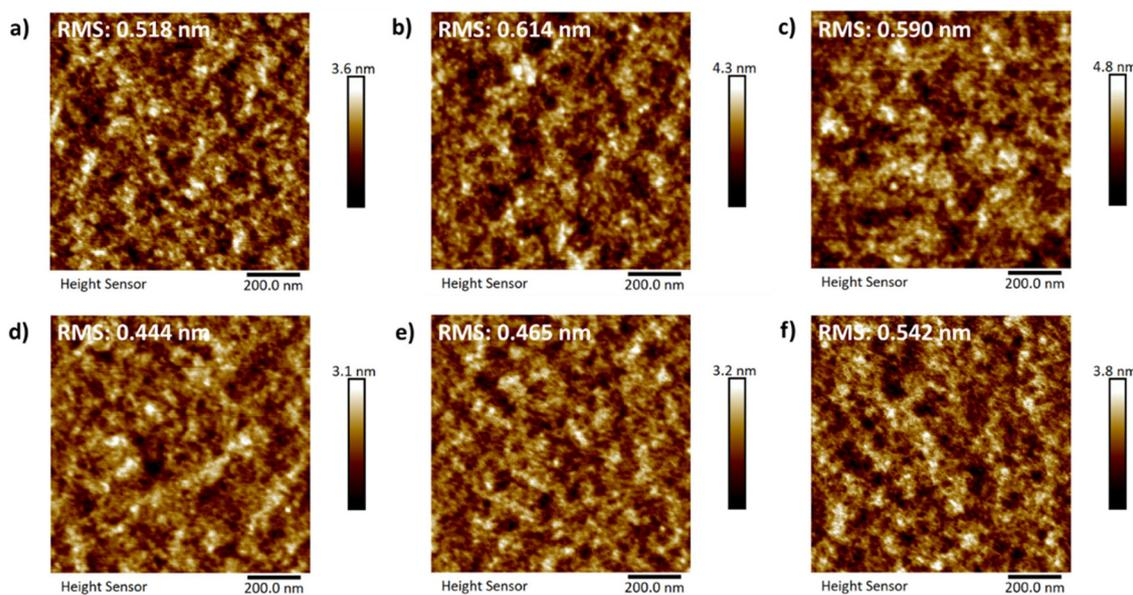
Fig. 3 Atomic force microscopy (AFM) height images with root-mean-square (RMS) surface roughness for *a*-P(iIT)-OH thin films casted from (a) chlorobenzene, (b) *o*-anisole and (c) 20% v/v *o*-anisole/*n*-BuOH; *a*-P(iIT)-TBS thin films casted from (d) chlorobenzene, (e) *o*-anisole and (f) 20% v/v *o*-anisole/*n*-BuOH. Scale bar is 200 nm.
