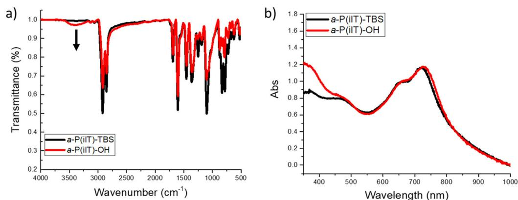
**Fig. 1** Fourier-Transform infrared (FTIR) spectra of (a) *a*-P(iIT)-TBS and *a*-P(iIT)-OH in the solid-state, and (b) UV-vis spectra of *a*-P(iIT)-TBS and *a*-P(iIT)-OH thin films casted on SiO<sub>2</sub>.
