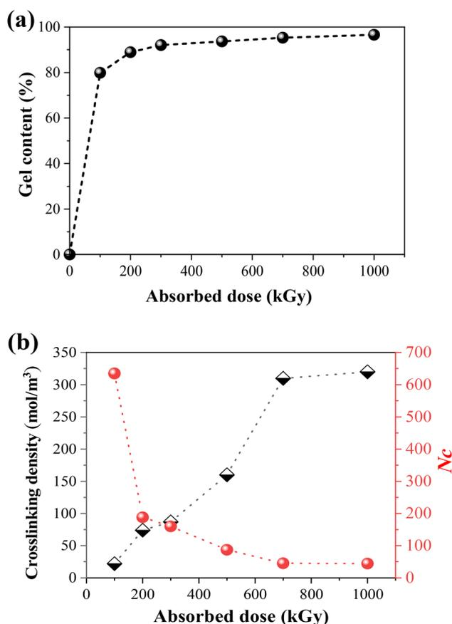
Fig. 2 (a) The gel content of irradiated TPI under an  $N_2$  atmosphere with different absorbed doses; (b) change of crosslinking density and monomer numbers between crosslinking points as a function of absorbed dose.
