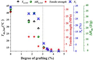
Fig. 11 A plot of  $T_{\rm m}$ ,  $\Delta H_{\rm m}$ , tensile strength, and  $X_{\rm c}$  as a function of grafting degree.
