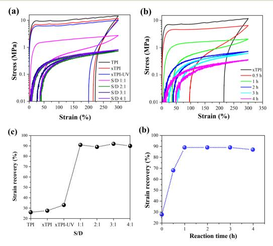
Fig. 10 Stress-strain curves of strain recovery tests (a) TPI samples with different S/D ratios (reaction time: 2 h); (b) q-xTPI with different reaction times (S/D = 2:1). The strain recovery of the TPI samples (c) with different S/D ratios and (d) with different reaction times.
