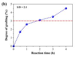
Fig. 4 The grafting degree of g-xTPI as a function of (a) S/D ratio and (b) reaction time.
