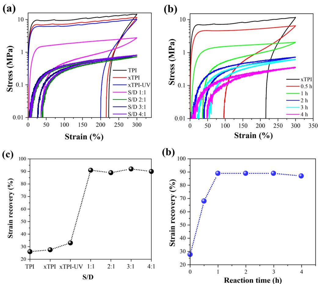
**Fig. 10** Stress–strain curves of strain recovery tests (a) TPI samples with different S/D ratios (reaction time: 2 h); (b) g-xTPI with different reaction times (S/D = 2 : 1). The strain recovery of the TPI samples (c) with different S/D ratios and (d) with different reaction times.
