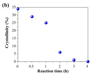
Fig. 8 The crystallinity of the modified xTPI (without heat treatment): (a) samples with the varied S/D ratio and fixed reaction time (2 h); (b) samples with different reaction times and a fixed S/D ratio (2:1).
