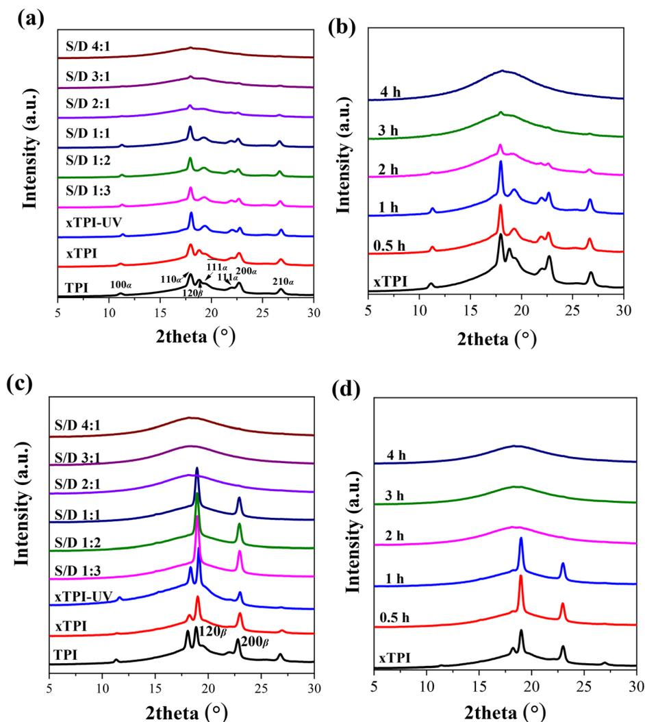
**Fig. 7** WAXS of the modified xTPI: (a) and (c) samples with the varied S/D ratio and fixed reaction time (2 h); (b) and (d) samples with different reaction times and fixed S/D ratio (2 : 1). The thermal history of the samples is different: (a) and (b) are as prepared samples; (c) and (d) are samples that melted at 120 °C and cooled to  $-40$  °C at  $10$  °C  $\text{min}^{-1}$  (for details, see the Experimental section). All the WAXS curves were taken at room temperature.
