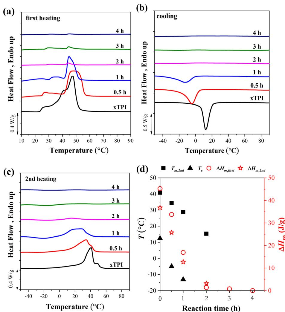
**Fig. 6** The DSC curves of g-xTPI with different reaction times and a fixed S/D ratio (2 : 1): (a) the first heating, (b) cooling, and (c) the second heating curves. (d)  $T_m$ ,  $T_c$  and  $\Delta H_m$  as a function of reaction time. The heating/cooling rate is  $10 \text{ }^\circ\text{C min}^{-1}$ .
