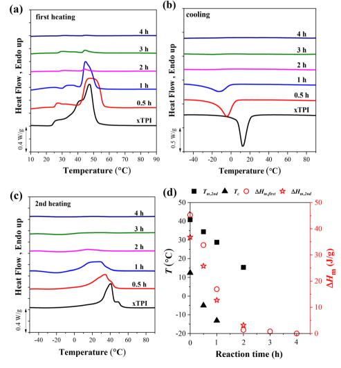
Fig. 6 The DSC curves of g-xTPI with different reaction times and a fixed S/D ratio (2:1): (a) the first heating, (b) cooling, and (c) the second heating curves. (d)  $T_{\rm mr}$ ,  $T_{\rm c}$  and  $\Delta H_{\rm m}$  as a function of reaction time. The heating/cooling rate is 10 °C min<sup>-1</sup>.
