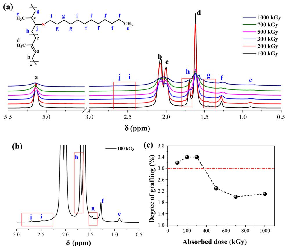
Fig. 3 (a) The <sup>1</sup>H-NMR spectra of the modified xTPI vary with absorbed doses (fixed S/D 3:1, reaction time 2 h); (b) magnified spectrum of xTPI with absorbed dose = 100 kGy; (c) the grafting ratio of the modified xTPI as a function of absorbed dose.
