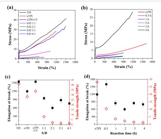
Fig. 9 The engineering stress-strain curves of q-xTPI with (a) different S/D ratios with a fixed reaction time (2 h) and (b) different reaction times with a fixed S/D ratio (2:1). The plots of elongation at break and tensile strength as a function of (c) S/D ratio and (d) reaction time.
