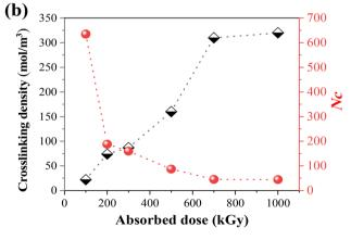
Fig. 2 (a) The gel content of irradiated TPI under an N2 atmosphere with different absorbed doses; (b) change of crosslinking density and monomer numbers between crosslinking points as a function of absorbed dose
