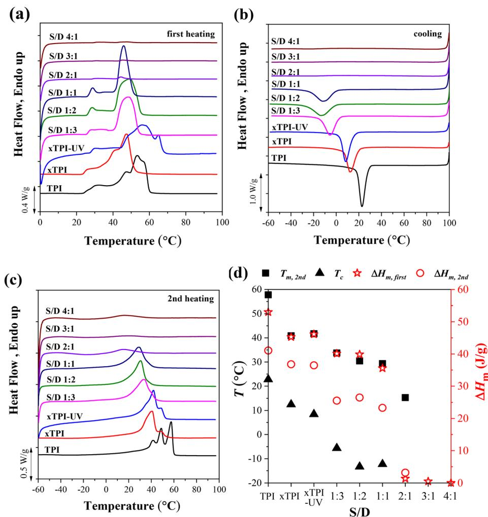
**Fig. 5** The DSC curves of the modified xTPI with fixed reaction time: (a) the first heating, (b) cooling, and (c) the second heating DSC curves. (d)  $T_m$ ,  $T_c$ , and  $\Delta H_m$  as a function of S/D. The heating/cooling rate is 10 °C min<sup>-1</sup>. The UV irradiation time was fixed at 2 h.
