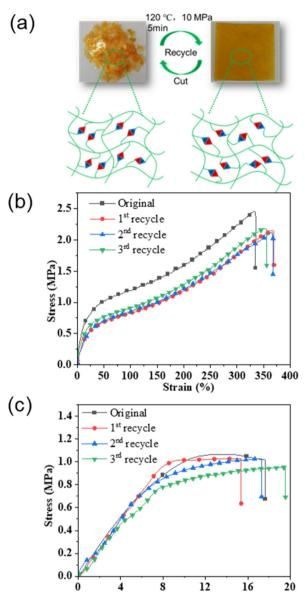
Fig. 4 Schematic representation of reprocessing of vitrimer (a); tensile test of FDV-1071 (b) and SCV-1071 (c).
