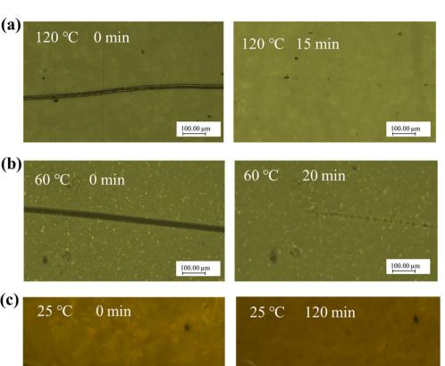
Fig. 7 Optical microscopy images of scratched FDV-1071 (a) at 120 °C, (b) at 60 °C, and (c) at 25 °C.
