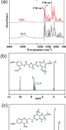
Fig. 2 FTIR spectra (a) and <sup>1</sup>H NMR spectra of FDV (b) and SCV (c).
