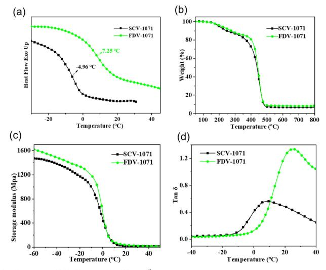
Fig. 5 DSC measurement (a), TGA (b), and DMA (c) and (d) of the 1<sup>st</sup> recycled vitrimers.
