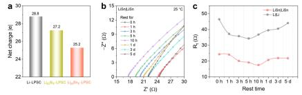
Fig. 1 (a) Net charges of Li/Li alloys and LPSC SE obtained from AIMD simulations. (b) Nyguist plots of LiSn|LiSn cells, demonstrating the evolution of cell impedance over varying rest times. (c) Changes in  $R_t$  for LiSn|LiSn and Li|Li cells as a function of rest time.
