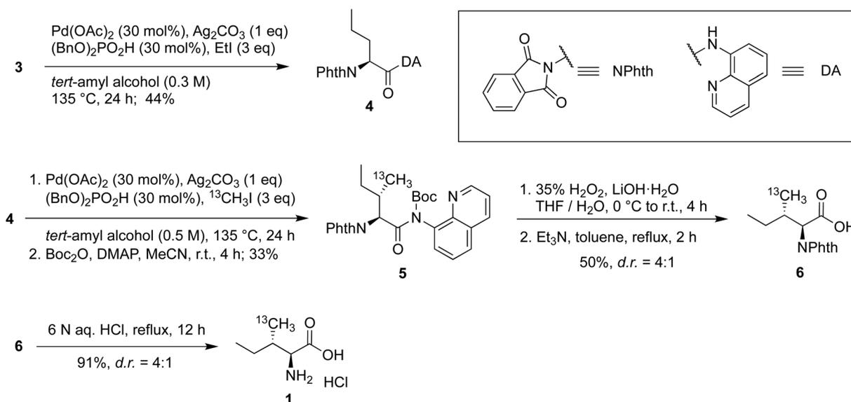
Scheme 2 Synthesis of  $^{13}\text{C}$  methyl-labeled  $\gamma$ 2-Ile-HCl (**1**).
