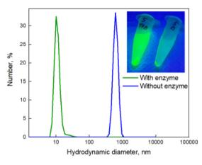
**Fig. 2** DLS data and image under UV lamp (insert) of the trehalose functionalised QDs after incubation with trehalase and centrifugation during 5 min at 15 000 R min<sup>-1</sup> (green line, corresponding to the left eppendorf in insert), and negative control (blue line, corresponding to the right eppendorf in insert).
