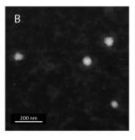
**Fig. 3** STEM images of (A) QDs after incubation with trehalase and centrifugation during 5 min at 15 000 R min<sup>-1</sup> and (B) the trehalose functionalized QDs in aggregates (negative control).
