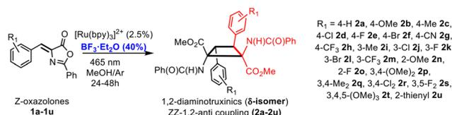
Fig. 3 Synthesis of delta isomers of cyclobutanes **2a–2u** (1,2-diaminotruxinic esters) by the [2 + 2]-photocycloaddition of (*Z*)-oxazolones **1a–1u** in the presence of BF<sub>3</sub>.
