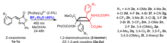
Fig. 3 Synthesis of delta isomers of cyclobutanes 2a–2u (1,2-diaminotruxinic esters) by the [2 + 2]-photocycloaddition of (Z)-oxazolones 1a–1u in the presence of BF 3 .
