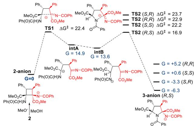
Fig. 12 Mechanism of the ring expansion of cyclobutanes **2** to give pyrrolidines **3**.
