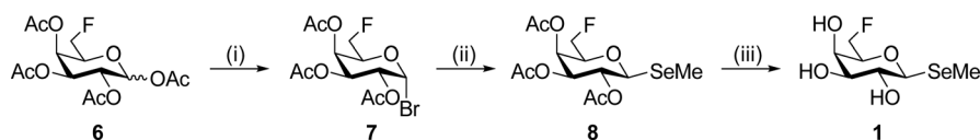
Scheme 1 Reagents and conditions: (i) HBr (33% in AcOH), CH 2 Cl 2 , RT, 2 h, 94%; (ii) (CH 3 ) 2 Se 2 , NaBH 4 , EtOH/CH 3 CN, RT, 22 h, 40%; (iii) NaOMe/MeOH, RT, 17 h, 83%.
