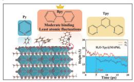
A moderate intensity ligand works best: a theoretical study on passivation effects of pyridine-based molecules for perovskite solar cells
