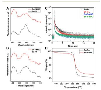
Fig. 3 The phosphorescence spectra (A and B) and lifetime (C) of Br-R/ S-L and Br-R/S-MOC films (D) the TGA polt of Br-R-L and Br-R-MOC.
