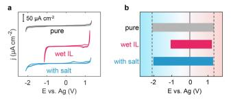
Fig. 5 Electrochemical windows for electrolytes. (a) Cyclic voltammograms of HOPG in pure [Emim][TFSI], wet [Emim][TFSI] and wet [Emim][TFSI] upon adding a salt. Scan rate: 100 mV s<sup>-1</sup>. Electrochemical windows for pure [Emim][TFSI], wet [Emim][TFSI] and wet [Emim][TFSI] upon adding a salt. The cathodic and anodic limits were determined according to a cut-off of  $\pm 30 \, \mu A \, cm^{-2}$ .
