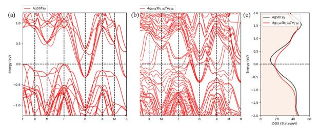
Fig. 4 Electronic band structure comparison of (a) pristine AgSbTe<sub>2</sub> and (b) the Ag<sub>2</sub>Te-deficient Ag<sub>1-x</sub>Sb<sub>1+x</sub>Te<sub>2+x</sub> composition. (c) Total density of states (DOS) showing higher DOS near the Fermi level for  $Ag_{1-x}Sb_{1+x}Te_{2+x}$ . The calculations were based on the conventional cell.
