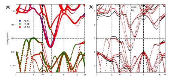
Fig. 5 Electronic band structures showing (a) the flatband of AgSbTe<sub>2</sub> with contributions from each element and (b) the effect of lattice parameters on the band position and the effective band gap. Both calculations were based on primitive cells.
