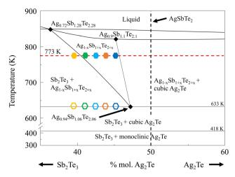
Fig. 1 Phase diagram of AgSbTe2, plotted as a fractional %mol of Sb<sub>2</sub>Te<sub>3</sub> and Ag<sub>2</sub>Te. Symbols of distinct colors represent the composition and processing temperature of the respective samples used in this study. Filled hexagon symbols represent samples annealed at 773 K for 24 hours followed by air quenching. Hollow hexagon symbols represent samples without such an annealing process. The figure is replotted from ref. 47
