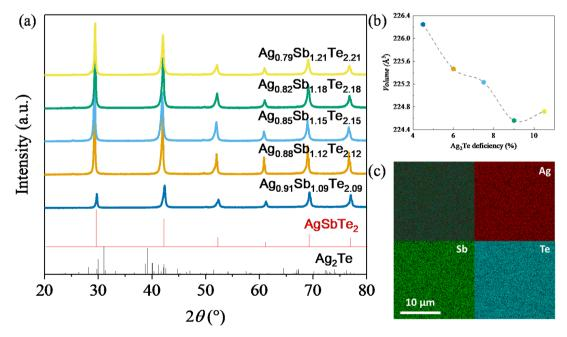
Fig. 2 Structural analysis of samples with various levels of Ag<sub>2</sub>Te deficiency. (a) XRD (X-ray diffraction) showing the absence of Ag<sub>2</sub>Te peaks in all samples. (b) Lattice parameters of all samples showing a decreasing trend with increasing Ag<sub>2</sub>Te deficiency. (c) SEM EDS analysis showing a homogeneous distribution and absence of Ag-rich nanoprecipitates.
