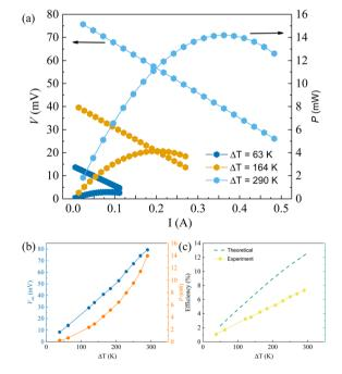
Fig. 7 Single leg power harvesting characteristics of Ag<sub>0.91</sub>Sb<sub>1.09</sub>Te<sub>2.09</sub> showing (a) voltage vs. current and output power vs. current, (b) open circuit voltage vs. temperature gradient and the corresponding maximum output power, and (c) theoretical and experimental power conversion efficiency as a function of temperature gradient.
