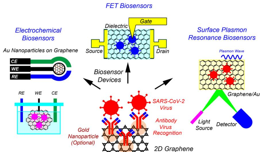
**Scheme 1** Schematic overview of graphene-based biosensors: electrochemical, field-effect transistor (FET), and surface plasmon resonance (SPR) sensors. Here, 'WE', 'RE', and 'CE' represent the working electrode, reference electrode, and counter electrode, respectively.
