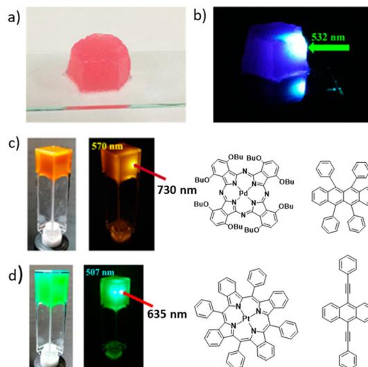
**Fig. 6** (a) DPA + PtOEP in an LBG gel matrix under normal light and (b) when irradiated with a 532 nm laser. (c and d) Generalization of the method with UC in LBG/rubrene/PdPc(OBu)<sub>8</sub> and LBG/BPEA/PtTPBP gels, respectively. Adopted with permission from ref. 37. Copyright 2015, American Chemical Society.
