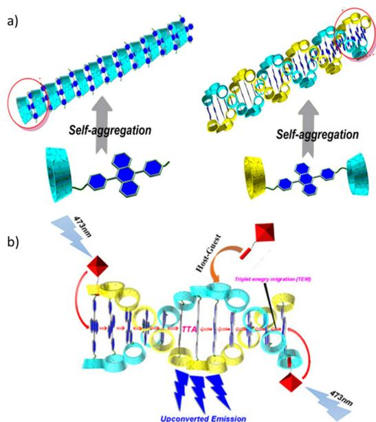
**Fig. 2** (a) Supramolecular self-assembled structure of fluorescent emitter (DPA- $\gamma$ -CD) molecules in water and (b) sensitizer guest molecules hosted in CD cavities, leading to upconverted emission through the TTA-UC mechanism. Adopted with permission from ref. 72. Copyright 2018, Wiley-VCH Verlag GmbH & Co. KGaA, Weinheim.
