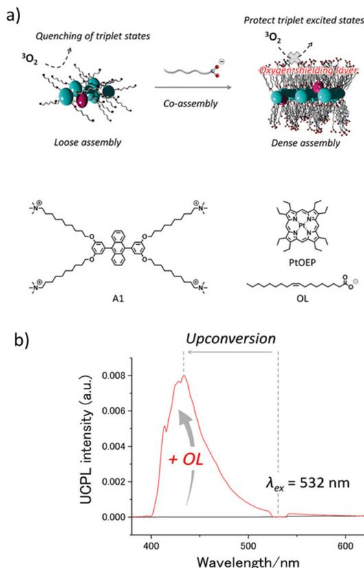
**Fig. 9** (a) Chemical structure of the functionalized DPA acceptor and scheme showing a co-assembled network that blocks the oxygen. (b) Plots showing the successful UC emission from the oleate–acceptor–PtOEP assembly and no UC from acceptor–PtOEP assembly in water. Adopted with permission from ref. 86. Copyright 2019, Wiley-VCH Verlag GmbH & Co. KGaA, Weinheim.
