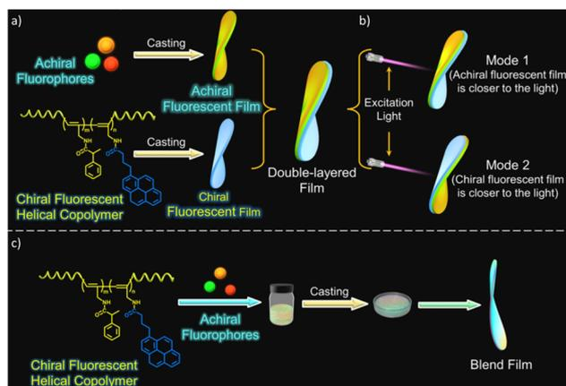
**Fig. 13** Schematic diagrams showing the formation of double layer film (a), two different modes of investigation with double layer film (b), and formation of blend films (c). Adopted with permission from ref. 144. Copyright 2023, American Chemical Society.
