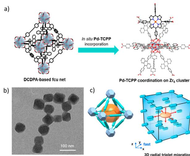
**Fig. 10** (a) Schematic diagram showing the preparation of a MOF containing an annihilator DCDPA and a sensitizer Pd-TCPP. (b) TEM image showing octahedral MOF structures. (c) Schematic design showing the three-dimensional triplet energy migration paths of the MOF. Adopted with permission from ref. 88. Copyright 2018, American Chemical Society.
