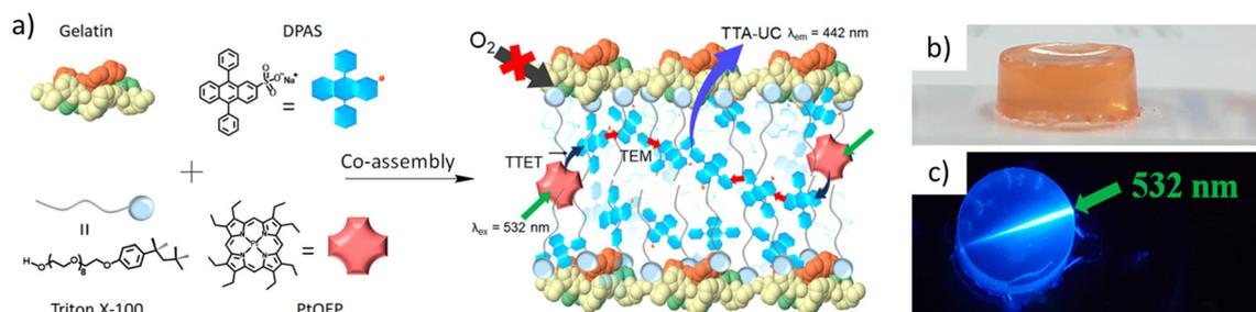
**Fig. 8** (a) Scheme showing the formation of a UC pair-surfactant-gelatin co-assembly in water and (b and c) a co-assembled hydrogel in normal light and upon irradiation with a 5432 nm laser. Adopted with permission from ref. 85. Copyright 2018, American Chemical Society.
