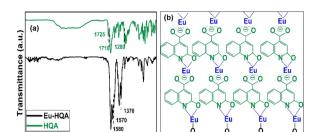
**Fig. 3** (a) FTIR spectra for HQA precursor powder and a representative Eu-HQA thin film sample. (b) Schematics of the anticipated film growth mode/bonding scheme in our Eu-HQA films.
