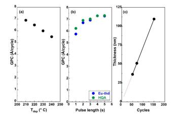
Fig. 2 Eu-HQA process optimization: (a) decrease of GPC with increasing deposition temperature; (b) increase and saturation of GPC upon increasing the pulse lengths of the two precursors separately ( $T_{\rm dep}=210$  °C; the other precursor pulse length fixed at 4 s); (c) linear dependence of film thickness on the number of ALD/MLD cycles applied ( $T_{\rm dep}=210$  °C; precursor/purge sequence = 4 s Eu(thd)<sub>3</sub>/6 s N<sub>2</sub>/4 s HQA/6 N<sub>2</sub>).
