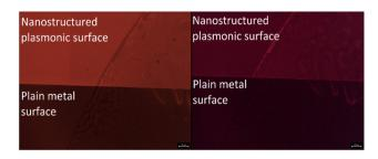
Fig. 5 Fluorescence microscope images: (left) 615 nm Eu<sup>3+</sup> emission, and (right) 660 nm FRET emission, obtained for Eu-HQA + Alexa647 surfaces on nanostructured plasmonic surface (top) and on plain metal surface (bottom). The tilted lines in the images represent the left-side edge of the Alexa647 droplet.
