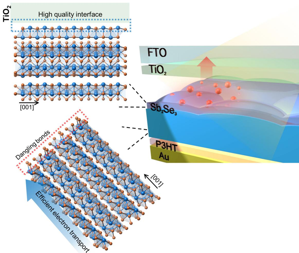
**Fig. 6** Schematic illustration of the proposed novel bilayer  $\text{Sb}_2\text{Se}_3$  configuration that can effectively transport the charge carriers without recombination and also form a high quality interface with the  $\text{TiO}_2$  layer.
