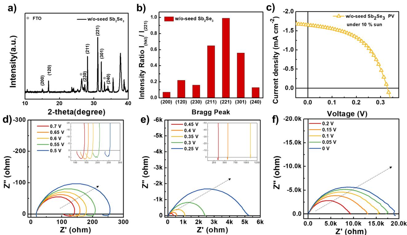
Fig. 4 (a) Diffraction patterns and (b) peak intensities ratio ( $I_{(hkl)}/I_{(221)}$ ) of the obtained w/o-seed Sb<sub>2</sub>Se<sub>3</sub> films (c)  $J$ - $V$  behavior exhibited by the w/o-seed Sb<sub>2</sub>Se<sub>3</sub> PV under 10% sun illumination. (d-f) Nyquist plots of the w/o-seed Sb<sub>2</sub>Se<sub>3</sub> PV at the designated applied potential.
