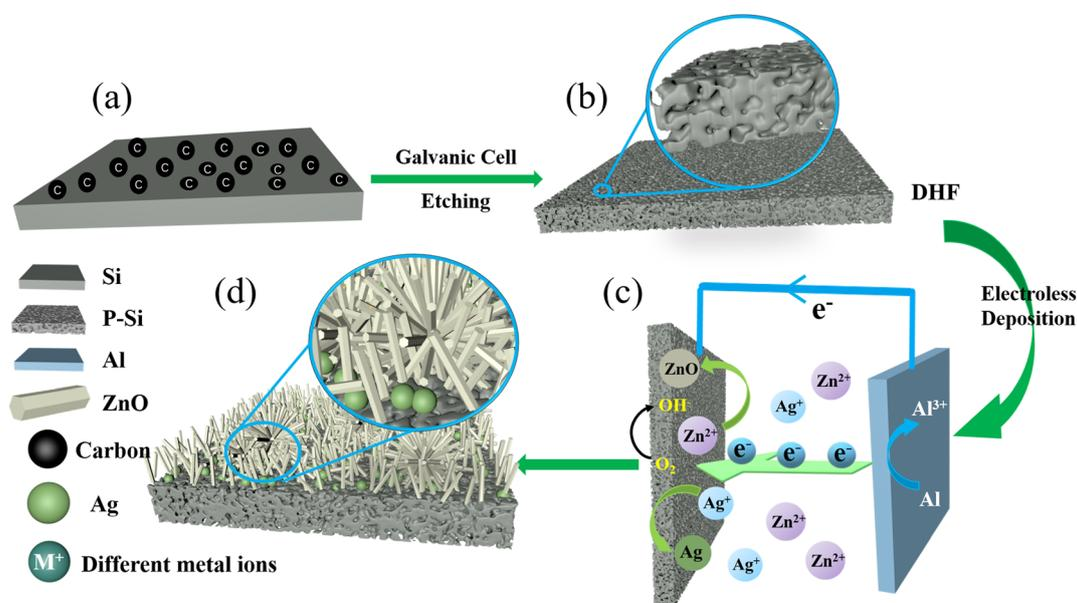
**Fig. 1** Synthesis process schematic of the P-Si/ZnO heterojunction. (a) Graphite particles are deposited and distributed on the surface of single-crystal silicon. (b) Three-dimensional structure diagram of P-Si. (c) Mechanism diagram of electroless deposition of ZnO on the porous silicon surface. (d) Three-dimensional structure diagram of the P-Si/ZnO heterojunction.
