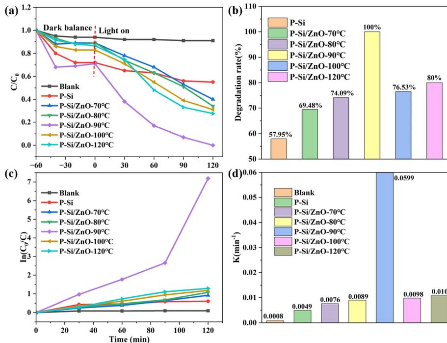
Fig. 5 Curves of photocatalytic degradation of RhB with different catalysts (a and b) and the apparent reaction rate constants ( $k$ ) (c and d). Experimental conditions: RhB, 5 mg L<sup>-1</sup>.
