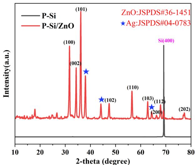
Fig. 2 XRD patterns of P-Si and P-Si/ZnO heterojunction.
