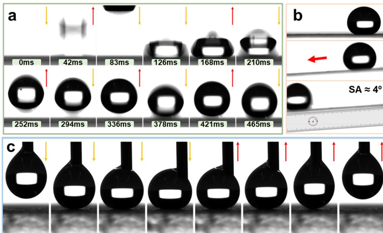
**Fig. 7** Analysis of dynamic behaviour of water droplets. (a) Images demonstrate the repeating bounce behavior of a  $15\ \mu\text{L}$  water droplet on a horizontally placed spray-coated glass. (b) The SA test result of AFSR/EP@n-SiO<sub>2</sub> coatings with a  $15\ \mu\text{L}$  water droplet. (c) The test process of non-stacking property of AFSR/EP@n-SiO<sub>2</sub> coatings towards the water droplet using a contact angle measuring instrument.
