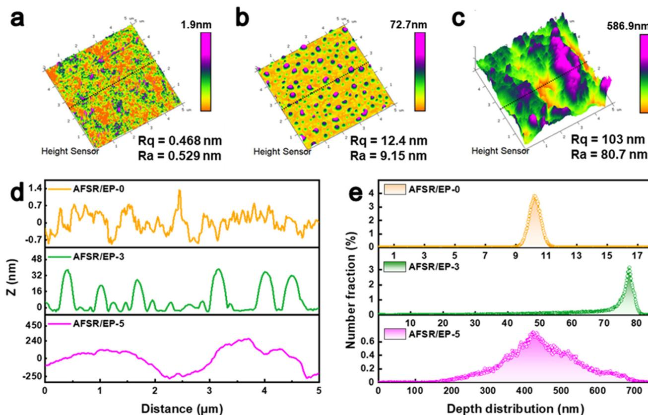
Fig. 3 Height-mode AFM images (scan area of  $5 \times 5 \mu\text{m}^2$ ) of AFSR/EP@n-SiO<sub>2</sub> coatings with different contents of n-SiO<sub>2</sub> particles, (a) n-SiO<sub>2</sub> = 0 wt%, (b) n-SiO<sub>2</sub> = 3 wt%, and (c) 5 wt%, respectively. (d) AFM 3D images showing the cross-sectional micro profiles at  $2.5 \mu\text{m}$  of the AFSR/EP@n-SiO<sub>2</sub> coating. (e) Statistical distribution of the height of the coating on the glass sheet substrate.
