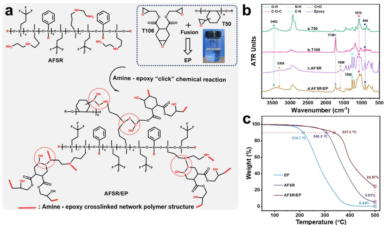
**Fig. 1** The chemical structure design of supramolecular silicone polymer. (a) Amine-epoxy “click” chemical reaction process and chemical structure, inset of (a) is an image of the mixture of T106 and T50, which has good transparency properties. (b) The ATR-FTIR spectra of modified polyfunctional group epoxy resin T50 and T106, self-synthesized amino fluor silicone resin AFSR, and supramolecular silicone polymer AFSR/EP. (c) TGA curves of EP, AFSR and AFSR/EP.
