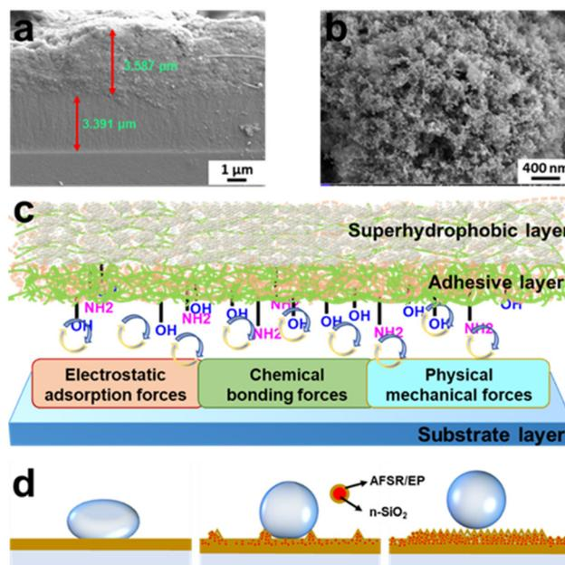
**Fig. 4** (a) FE-SEM image of double-layer cross-section surface of glass sample with coating. (b) High power FE-SEM image of the AFSR/EP@n-SiO<sub>2</sub> superhydrophobic coating surface at nanoscale magnifications. (c) Schematic diagram of the layered structure of the AFSR/EP@n-SiO<sub>2</sub> superhydrophobic coating and the mechanism of strong bonding properties, and (d) simplified wetting model of three rough coating structures and different hydrophobic mechanism diagrams.
