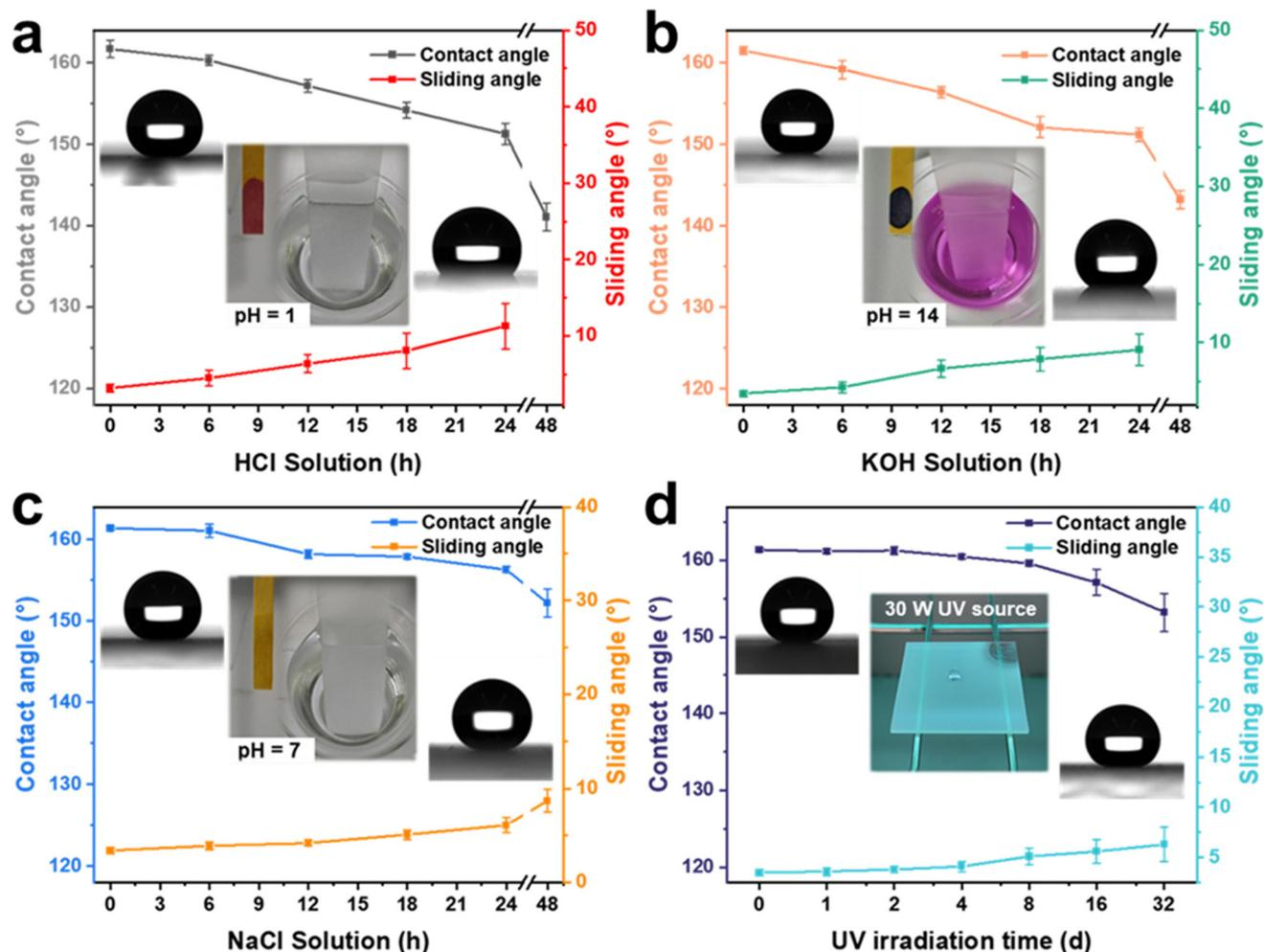
Fig. 6 Contact angle and sliding angle of AFSR/EP@n-SiO<sub>2</sub> coatings immersed in various harsh solutions with (a) pH = 1, HCl, (b) pH = 14, KOH, phenolphthalein indicator was added for color indication, and (c) pH = 7, NaCl (10 wt%) for a long time. (d) Hydrophobicity test of the prepared surface under 30 W ultraviolet light source.
