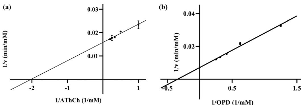
Fig. 8 Lineweaver-Burk plots of (a) RONS immobilized AChE and (b) MnO<sub>2</sub> nanozyme.
