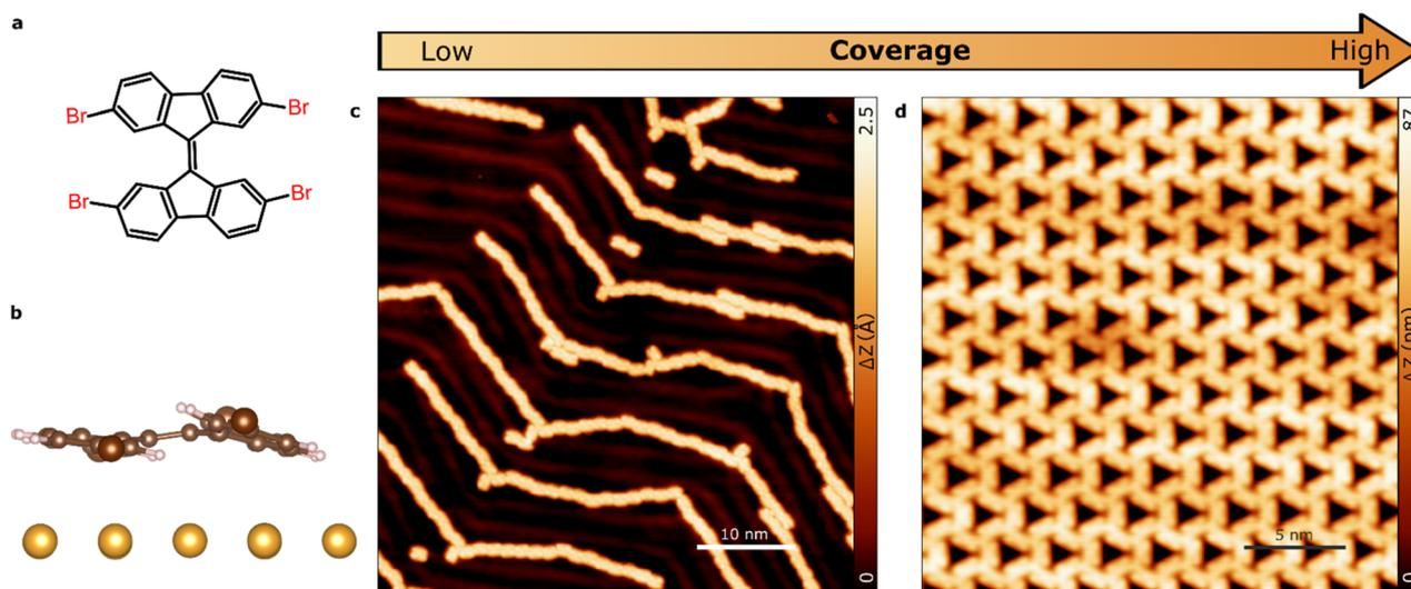
**Fig. 1** Supramolecular assembly of TBF molecule on Au(111). (a) Molecular model of the TBF. (b) Side view calculation of the relaxed TBF on the Au(111) surface. (c and d) STM topography overview after (c) low-, (d) high-coverage deposition at RT on Au(111). (c) (0.1 V; 10 pA) (d) (1.2 V; 0.1 nA).
