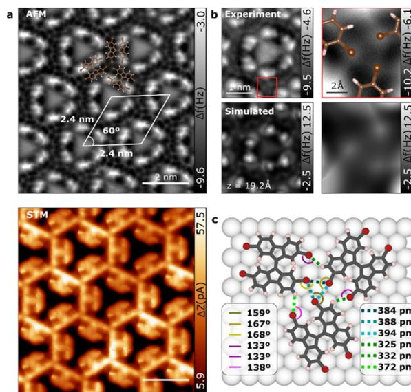
**Fig. 3** Characterization of the two-dimensional phase of TBF molecules on Au(111). (a) nc-AFM and STM constant height images of the hexagonal structure with a lattice of  $2.4 \text{ nm} \times 2.4 \text{ nm}$  with a superimposed ball-stick model of three TBF molecules. (b) Experimental (top) and simulated (down) nc-AFM images of a close-up view of the center of the pore (left) and the Br...Br bond (right) of the TBF molecules. (c) DFT model of the relaxed TBF molecules on Au(111) surface.
