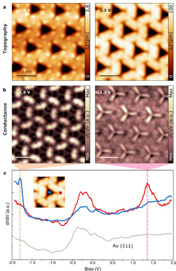
**Fig. 5** Electronic characterization of the 2D supramolecular structure. (a) STM topography overview images acquired at  $-1.8$  V (left) and  $1.2$  V (right). (b) Differential conductance images of the 2D structure at the indicated voltages. (c)  $dI/dV$  spectroscopies at the positions marked with points in the inset image.
