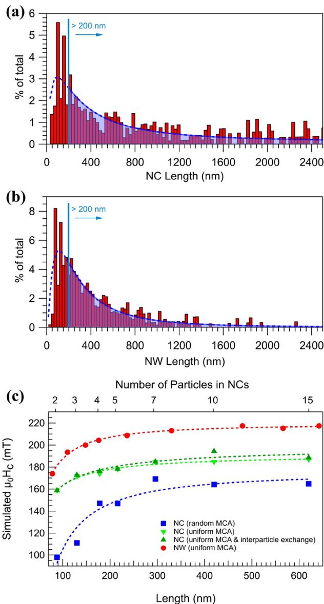
**Fig. 4** Histograms displaying the percentage of the total number of 1D structures (weighted by area) exhibiting a specific length for NCs (a) and NWs (b). The bottom axis shows calculated length assuming an average 40 nm diameter, the curves are guide to the eye. (c) Simulated coercivity values of NCs and NWs per length.
