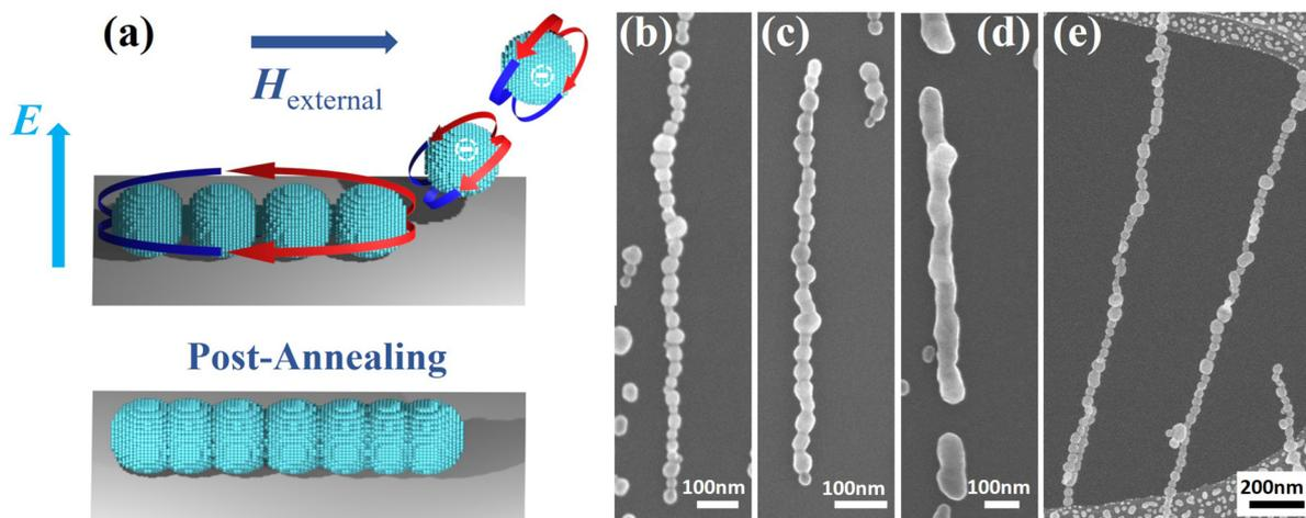
**Fig. 1** (a) Schematic illustration of NC formation by attracting negatively charged particles using an electric field  $\vec{E}$  from the gas phase and self-assembling them by employing an external magnetic field  $\vec{H}_{\text{external}}$ . (b) SEM images of an as-prepared NC, and post-annealed NWs at (c) 673 and (d) 773 K. (e) Free-standing NCs deposited on a TEM grid.
