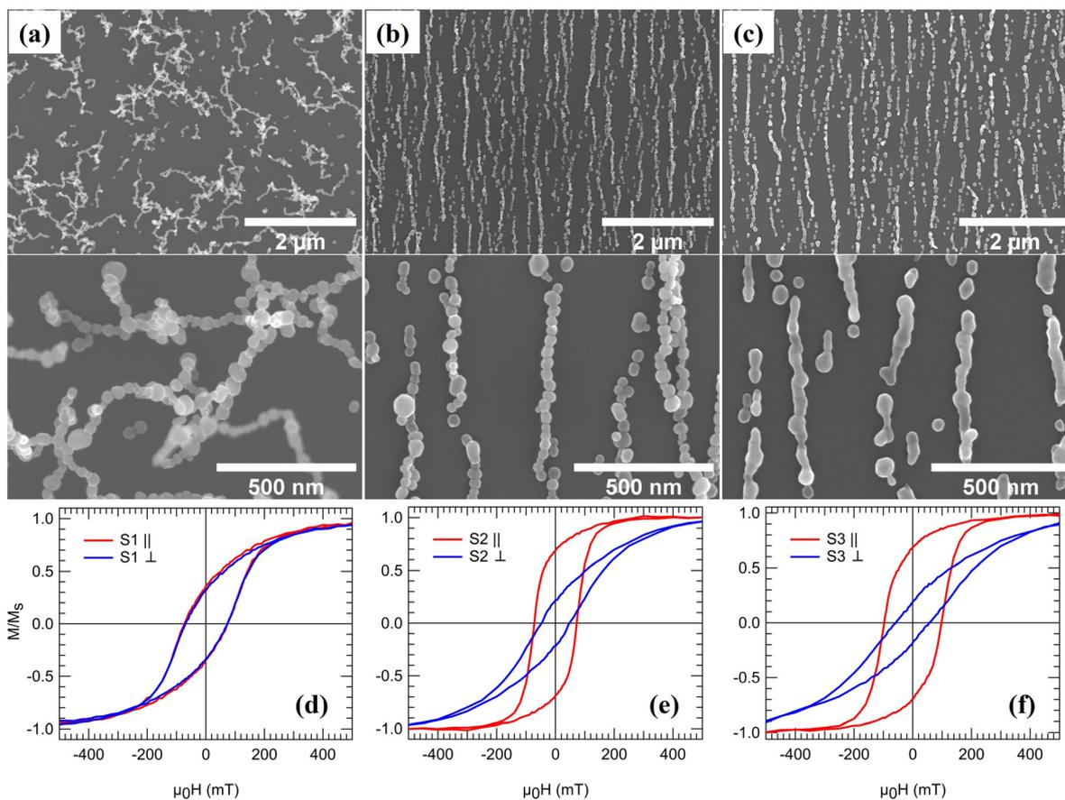
**Fig. 3** SEM images of (a) randomly oriented interconnected chains, S1, (b) ordered NCs, S2, and (c) continuous NWs, S3, on quartz substrates. Magnetic hysteresis loops of (d) S1, (e) S2, and (f) S3 measured with an in-plane magnetic field oriented parallel (||) and perpendicular (⊥) to the longitudinal direction of the NCs and NWs.
