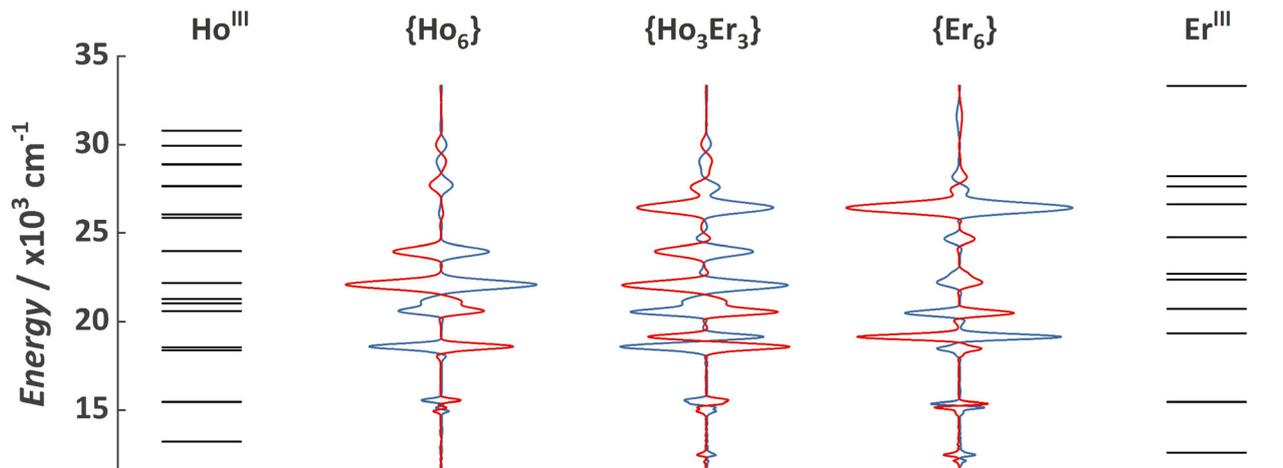
Fig. 2 Energy level diagram showing the excited states of  $\text{Ho}^{\text{III}}$  and  $\text{Er}^{\text{III}}$  and MCD spectra for  $\{\text{Ho}_6\}$ ,  $\{\text{Ho}_3\text{Er}_3\}$ , and  $\{\text{Er}_6\}$  MCAs obtained under an applied magnetic field of 1.0 T (blue lines) and  $-1.0$  T (red lines). Energy levels were obtained in Carnall book<sup>35</sup> and are summarized in Table S1.†
