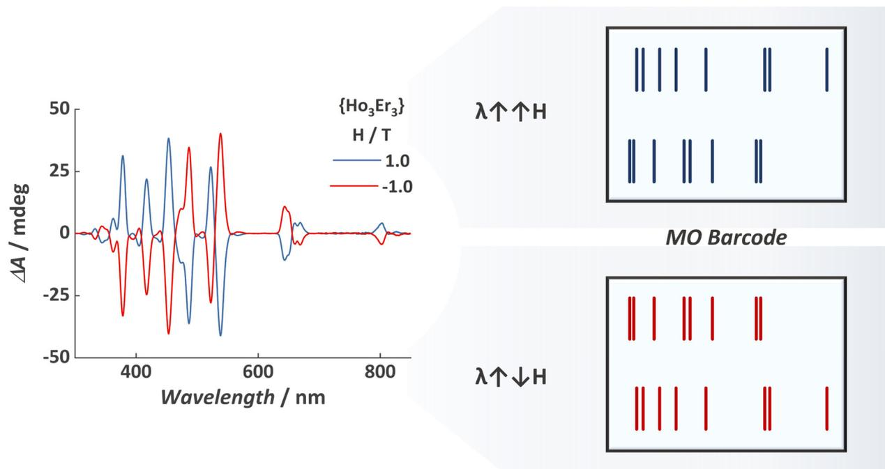
Fig. 3 (Left) MCD spectra for  $\{\text{Ho}_3\text{Er}_3\}$  and (right) representation of the magneto-optical barcode read-out. For an overlay of the read-out representation and MCD spectra, see Fig. S4 and S5.†
