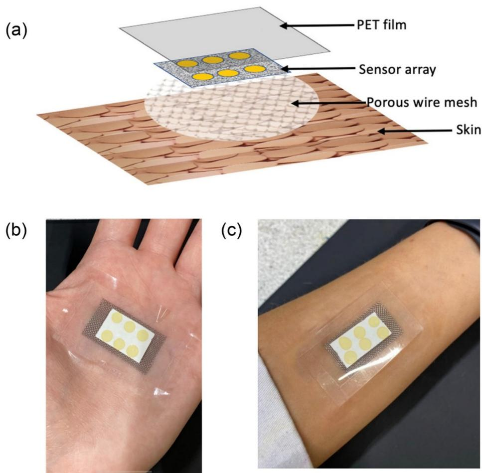
**Fig. 11** A BCG sol-gel dye-spotted cellulose substrate-based colorimetric wearable skin surface pH sensor. (a) Three layers of the sensor, (b) the sensor taped on a palm and (c) the sensor taped on the wrist [this figure has been reproduced from ref. 96 under open access article in terms of the Creative Commons CC-BY license].
