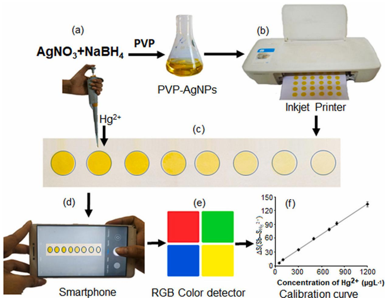
**Fig. 6** Systematic representation of the development of an AgNPs-PVP-based portable colorimetric sensor. (a) Synthesis of AgNPs-PVP. (b) Printing of AgNPs in filter paper. (c) Pipetting  $\text{Hg}^{2+}$  in an AgNP sensing probe. (d) Image captured using a smartphone. (e) RGB value analyzed using ImageJ software. (f) The result as a calibration curve [this figure has been reproduced from ref. 60 with permission from Elsevier Sciences, copyright 2021].
