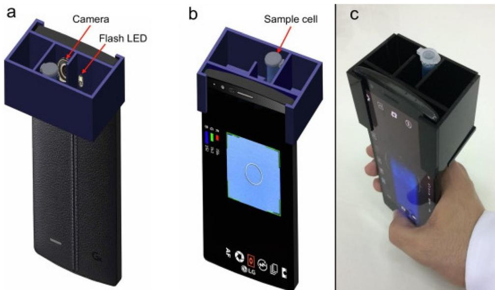
**Fig. 2** (a-c) show the portable handheld RGB-based colorimetry device for the self-referenced solution-based determination of the water content in ethanol [this figure has been reproduced from ref. 40 with permission from Elsevier Sciences, copyright 2020].
