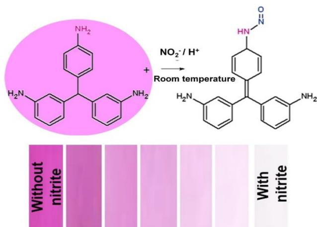
Fig. 4 Systematic representation of fuchsin dye-based nitrite ion (NO<sub>2</sub><sup>-</sup>) detection in real water and wastewater samples [this figure has been reproduced from ref. 49 with permission from Elsevier Sciences, copyright 2019].
