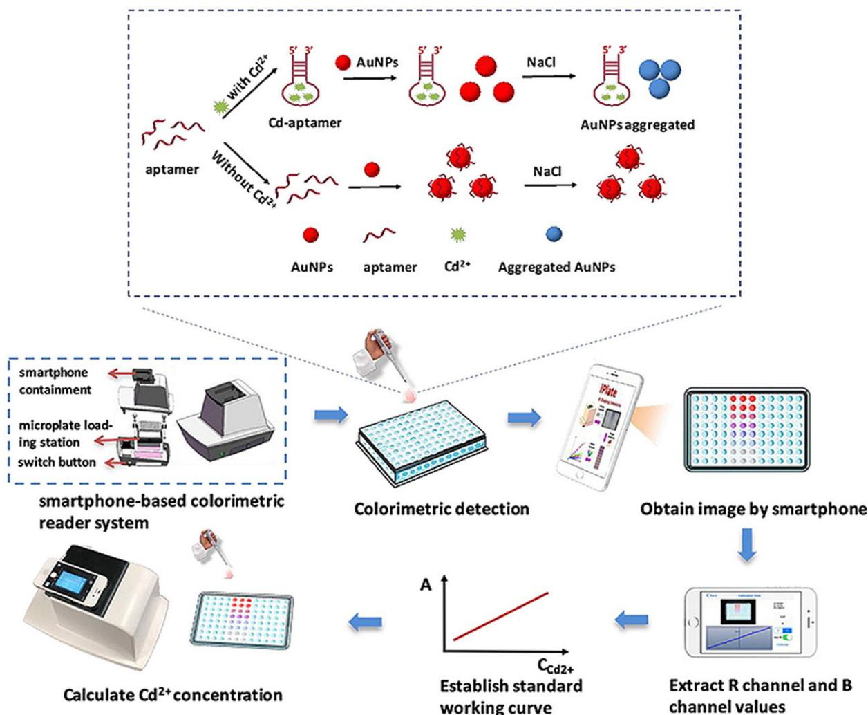
Fig. 5 Mechanism of the detection of  $\text{Cd}^{2+}$  in drinking water using an AuNP-aptamer based sensing probe [this figure has been reproduced from ref. 56 with permission from Elsevier Sciences, copyright 2020].
