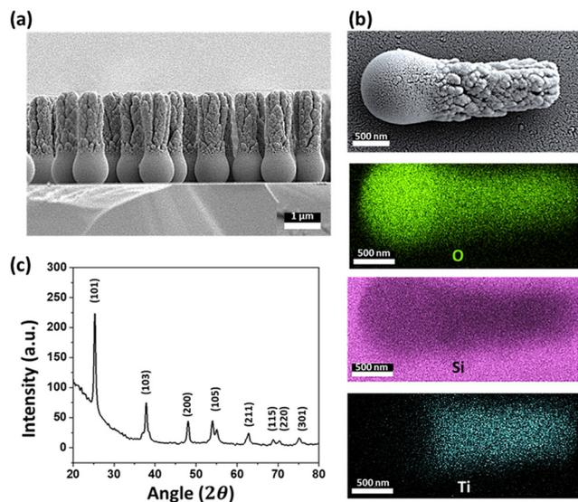
**Fig. 2** Characterization of rod-shaped micromotors. (a) Cross-sectional SEM view of micromotors. (b) EDX mapping showing the elemental distribution over fabricated micromotors. (c) XRD analysis shows the phase transformation of  $\text{TiO}_2$  after annealing.
