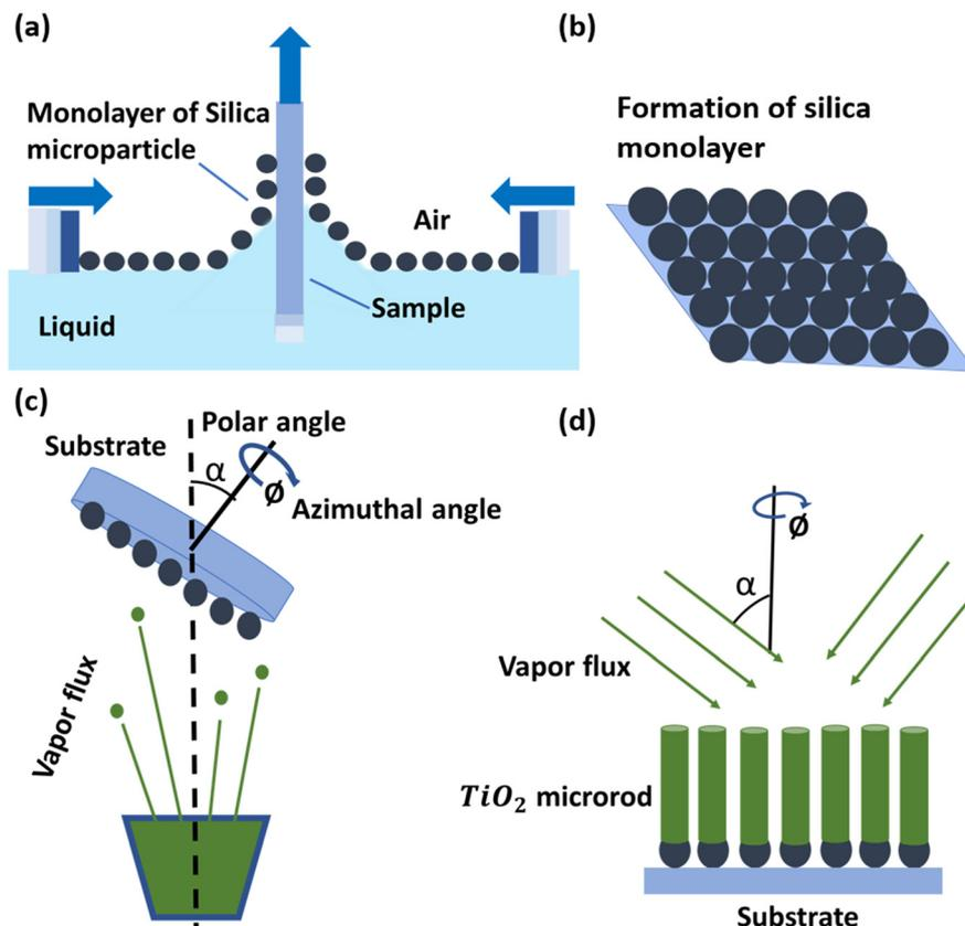
**Fig. 1** Fabrication of rod-shaped micromotors. (a) Schematic representation of the Langmuir Blodgett (LB) technique for the monolayer formation of silica microparticles. (b) Schematic of the silica microparticle monolayer over the Si substrate. (c) Schematic representation of rod formation by glancing angle deposition (GLAD) using the DSG technique. (d) Dynamic shadowing at a very high vapor incidence angle ( $\alpha$ ) on a rotating substrate leads to the growth of vertical rods.
