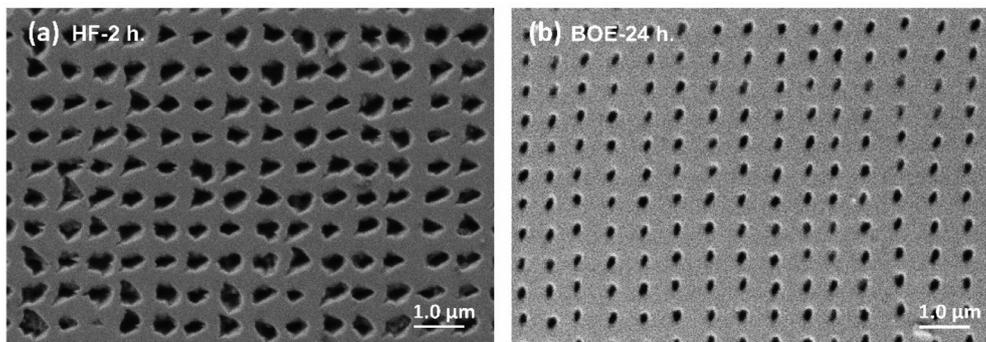
**Fig. 2** Comparison of the sample surface by using 40% HF (a) and BOE (b) in chemical etching. The pulse energy in prior laser writing is 11 nJ. The etching time is 2 hours and 24 hours for 40% HF and BOE, respectively.
