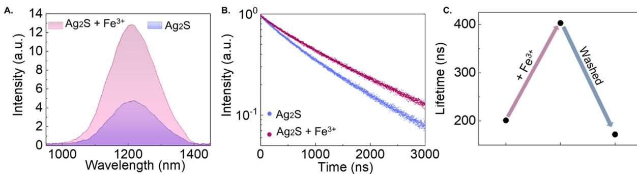
**Fig. 5** Effect of iron ions. (A) Emission spectra measured at 20 °C of Ag<sub>2</sub>S LNTs as synthesized and upon 2 μL of 1 mM FeCl<sub>3</sub> addition. (B) Lifetime measurements measured at 20 °C of Ag<sub>2</sub>S LNTs as synthesized and upon 2 μL of 1 mM FeCl<sub>3</sub> addition. (C) Lifetime values measured at 20 °C of Ag<sub>2</sub>S LNTs as synthesized, upon 2 μL of 1 mM FeCl<sub>3</sub> addition and after washing.
