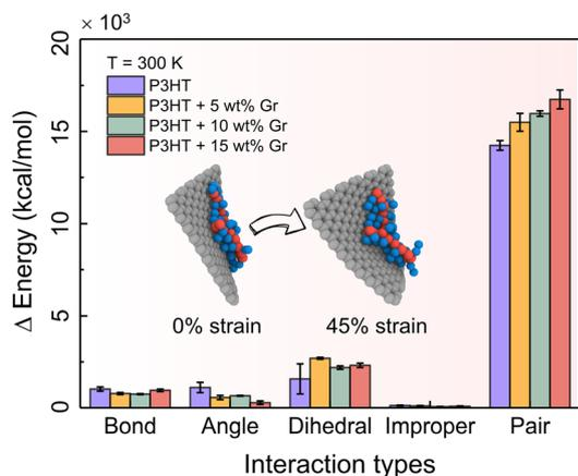
**Fig. 6** Energy changes of bonds, angles, dihedrals, improper and cohesive (*i.e.*, pair) terms between the deformed and nondeformed states for the pristine P3HT and P3HT/graphene nanocomposite systems with different graphene contents at  $T = 300$  K.
