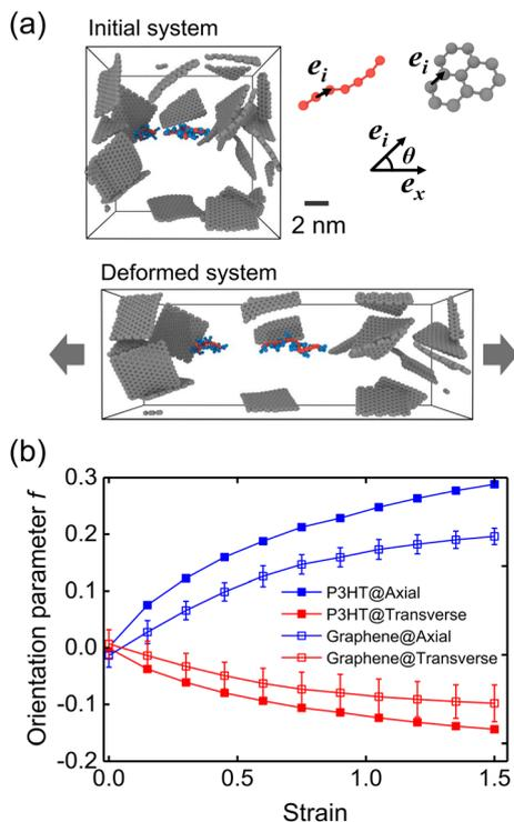
**Fig. 11** Strain-induced chain conformation of the P3HT/graphene nanocomposite with 5 wt% graphene content at 300 K. (a) Representative snapshot of amorphous morphology before and after straining to 150% (only graphene and two P3HT chains are shown for clarity). (b) Orientation parameter  $f$  of the axial and transverse components of the P3HT backbone and the graphene C–C bond during the uniaxial tension deformation at 300 K.
