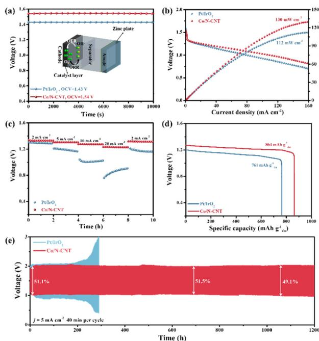
**Fig. 5** Performance of Co/N-CNT-assembled liquid ZABs: (a) open-circuit voltage plots (inset: schematic illustration of the assembled device), (b) polarization and power density curves, (c) galvanostatic discharge plots at different current densities, and (d) specific capacity at 5 mA cm<sup>-2</sup>, and (e) discharge/charge cycling plots of Co/N-CNT and Pt/IrO<sub>2</sub>.
