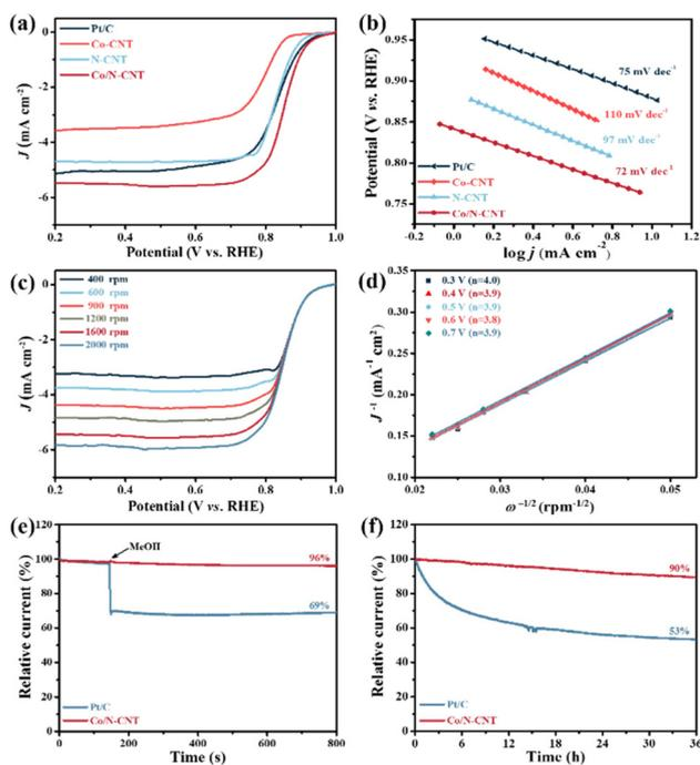
**Fig. 3** ORR performance of the as-crafted samples (*i.e.*, Co/N-CNT, Co-CNT, N-CNT and Pt/C) in 0.1 M KOH solution saturated with O<sub>2</sub>: (a) LSV curves, (b) Tafel slopes, (c) LSV plots of Co/N-CNT at various speeds, (d) Koutecky–Levich plots of Co/N-CNT at different voltages, (e) methanol resistance, and (f) the chronoamperometry *i*–*t* curves.
