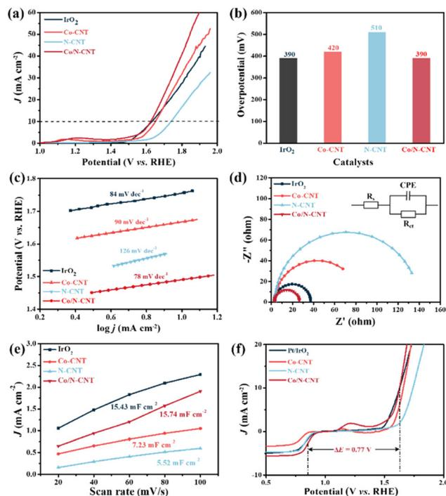
**Fig. 4** OER performance of the as-crafted samples (*i.e.*, Co/N-CNT, Co-CNT, N-CNT and IrO<sub>2</sub>) in 0.1 M KOH solution saturated with O<sub>2</sub>: (a) LSV curves, (b) OER overpotential at 10 mA cm<sup>-2</sup>, (c) Tafel slopes, (d) Nyquist plots, (e)  $C_{dl}$  values, and (f) integrated ORR/OER LSV curves.
