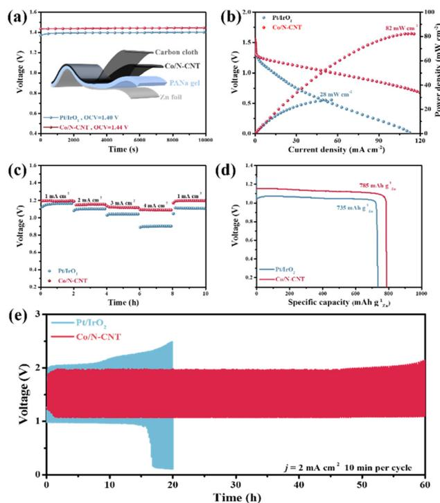
**Fig. 6** Performance of the home-made Co/N-CNT-based flexible ZABs: (a) open-circuit voltage plots (inset: schematic illustration of the flexible devices), (b) polarization and power density curves, (c) galvanostatic discharge plots at different current densities, and (d) specific capacity measured at a current density of 2 mA cm<sup>-2</sup>, (e) galvanostatic discharge/charge cycling of Co/N-CNT and Pt/IrO<sub>2</sub>.
