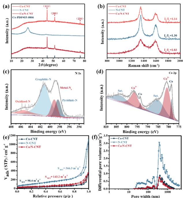
**Fig. 2** (a) XRD patterns, and (b) Raman analysis of Co/N-CNT, Co-CNT and N-CNT; high-resolution XPS analysis of (c) N 1s and (d) Co 2p of Co/N-CNT; (e)  $\text{N}_2$  adsorption/desorption curves, and (f) the pore size distribution of Co/N-CNT, Co-CNT and N-CNT.
