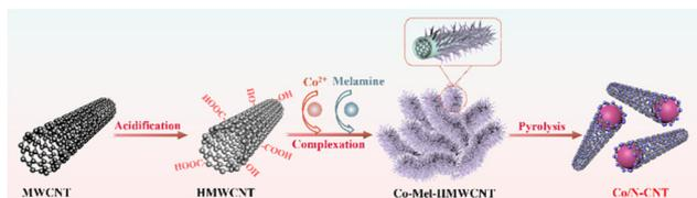
**Scheme 1** Schematic route to the Co/N-CNT electrocatalyst.
