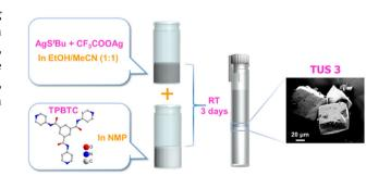
Fig. 1 Schematic illustration of the preparation route to TUS 3 single crystals. The SEM image of the obtained crystals is depicted in the magnified view.
