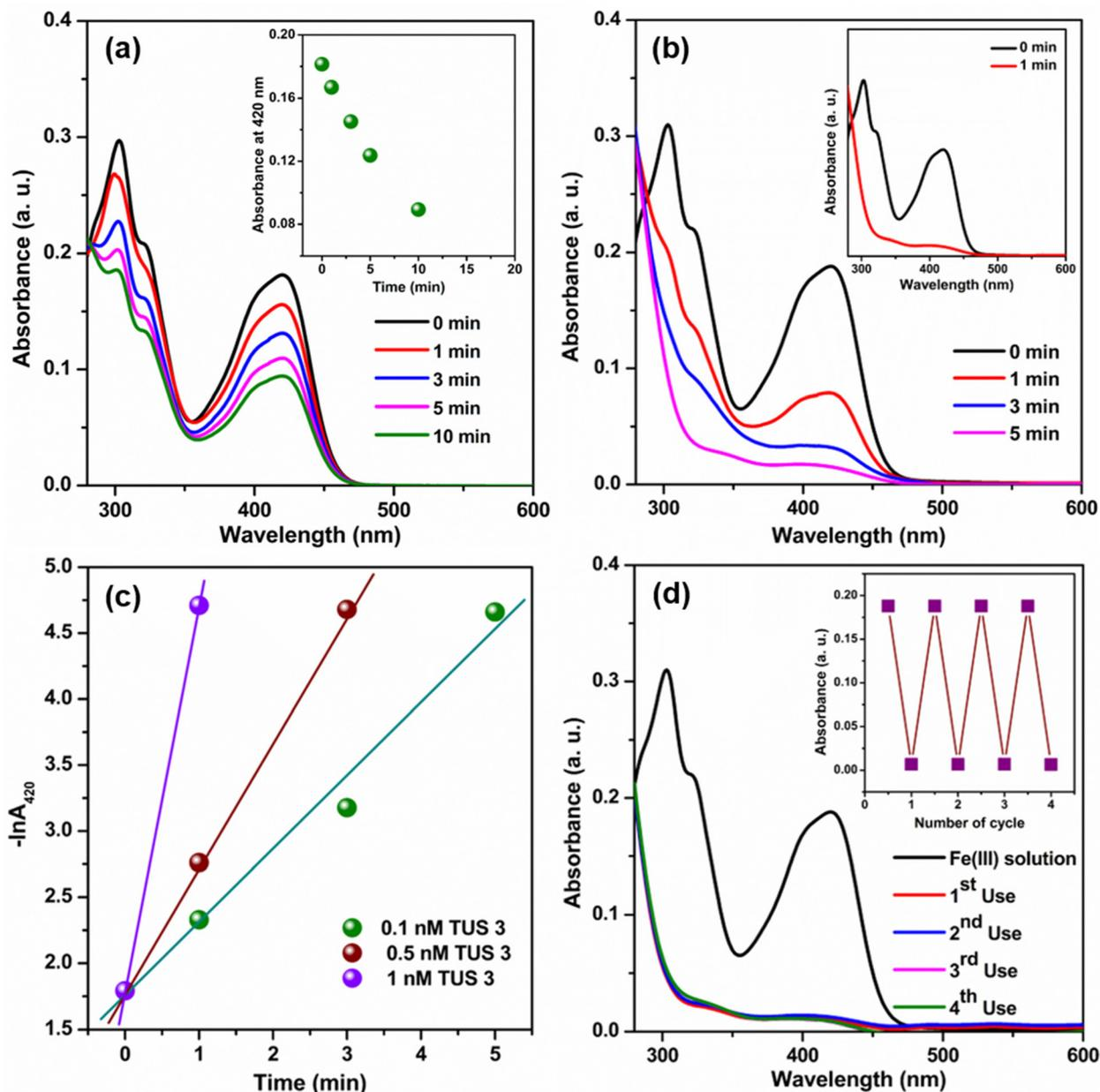
Fig. 6 (a) Reduction of Fe(III) in presence of  $\text{NaBH}_4$  with time, inset showing the absorbance at 420 nm against time, (b) effect of TUS 3 in this reaction with different concentrations, (c) and  $-\ln A_{420}$  against time when TUS 3 was added in different concentrations, and (d) reusability of TUS 3 up to 4<sup>th</sup> cycle.
