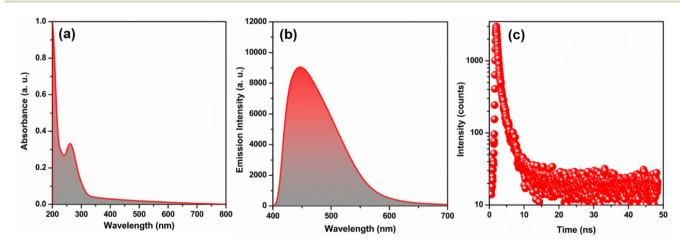
Fig. 5 (a) UV-Vis absorption spectrum of TUS 3 in water medium, (b) photoluminescence spectrum of TUS 3 in water medium excited at 330 nm, and (c) TCSPC histogram of TUS 3 at emission wavelength of 434 ± 0.80 nm.
