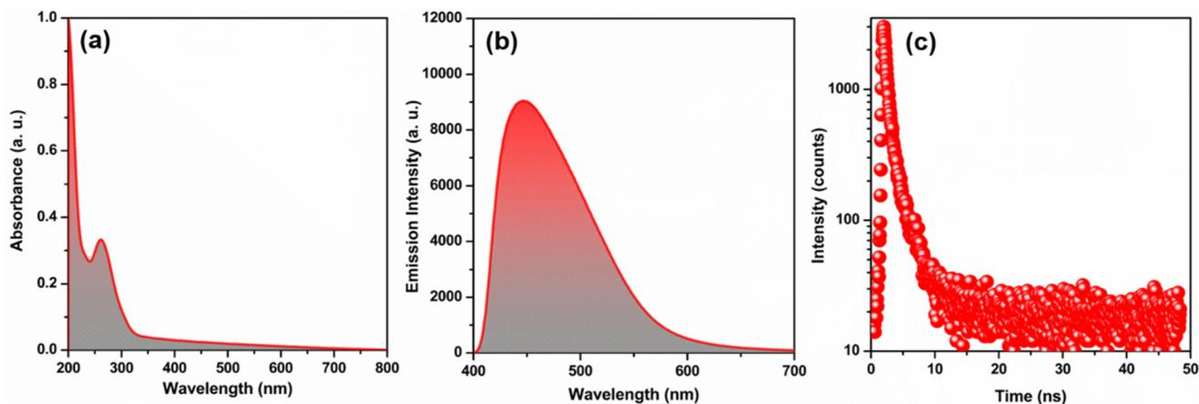
Fig. 5 (a) UV-Vis absorption spectrum of TUS 3 in water medium, (b) photoluminescence spectrum of TUS 3 in water medium excited at 330 nm, and (c) TCSPC histogram of TUS 3 at emission wavelength of  $434 \pm 0.80$  nm.
