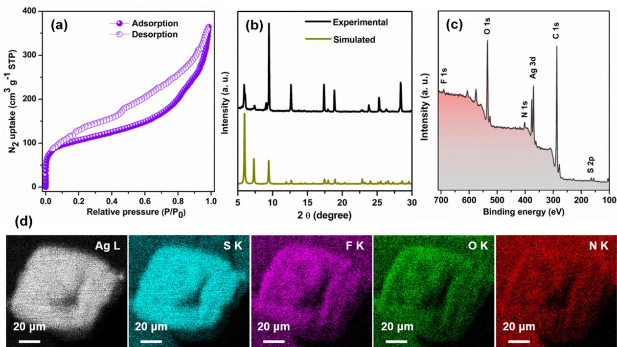
Fig. 4 (a) Nitrogen sorption isotherms of TUS 3, (b) simulated and experimental PXRD patterns of TUS 3, (c) XPS survey plot of TUS 3, and (d) SEM-EDS mapping of TUS 3 (individual elements are detected in each frame).
