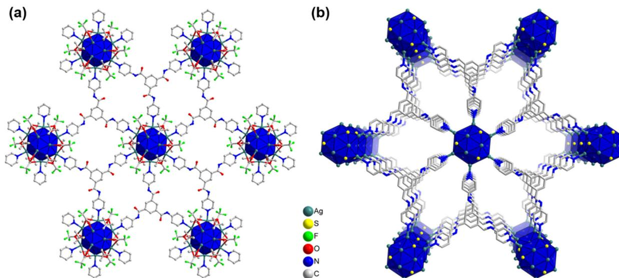
Fig. 3 (a) Planar 2D architecture of TUS 3 where  $\text{Ag}_{12}$  cluster nodes are linked with the linker molecules, (b) 3D architecture of TUS 3. For clarity, linker part occasionally and H atoms are omitted.
