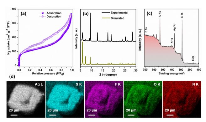
Fig. 4 (a) Nitrogen sorption isotherms of TUS 3, (b) simulated and experimental PXRD patterns of TUS 3, (c) XPS survey plot of TUS 3, and (d) SEM-EDS mapping of TUS 3 (individual elements are detected in each frame).
