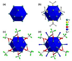
Fig. 2 Structural anatomy of TUS 3: (a) the geometry of Ag<sub>12</sub> cluster node, (b) connectivity of thiolate ligands, (c) connectivity of trifluoroacetate ligands, and (d) connectivity of linkers on the Ag<sub>12</sub> cluster node. For clarity, H atoms are always omitted, and occasionally the other ligand and linker parts are omitted.
