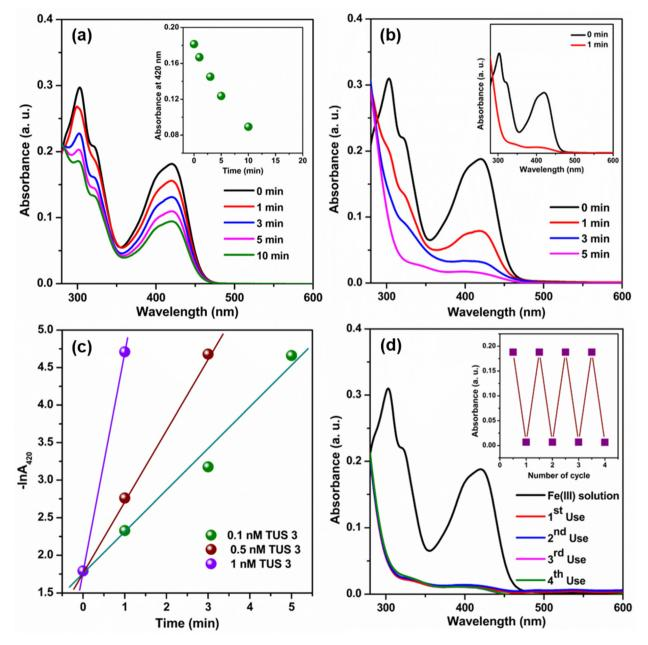
Fig. 6 (a) Reduction of Fe(III) in presence of NaBH<sub>4</sub> with time, inset showing the absorbance at 420 nm against time, (b) effect of TUS 3 in this reaction with different concentrations, (c) and  $-\ln A_{420}$  against time when TUS 3 was added in different concentrations, and (d) reusability of TUS 3 up to  $4^{th}$  cycle.
