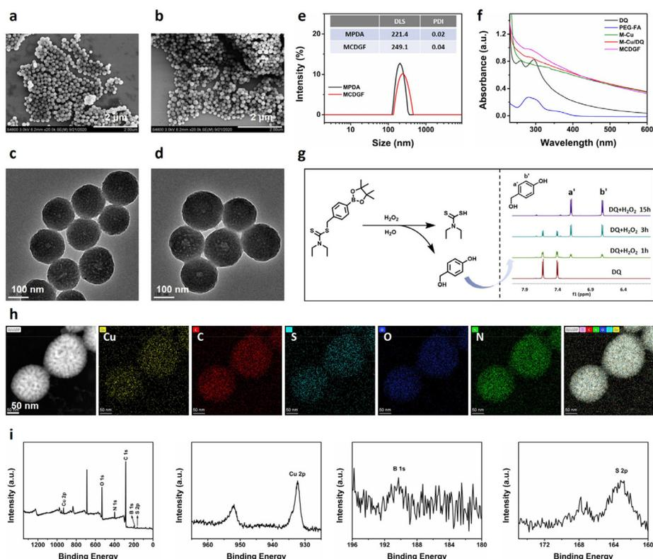
**Fig. 1** SEM images of (a) MPDA and (b) MCDGF. TEM images of (c) MPDA and (d) MCDGF. (e) DLS and PDI of nanoparticles in water. (f) UV-vis absorption spectra of different nanoparticles, free DQ and free FA/PEG. (g)  $^1\text{H}$  NMR spectral changes of DQ in the presence of  $\text{H}_2\text{O}_2$ . (h) Elemental mapping of MCDGF. (i) XPS results of MCDGF.
