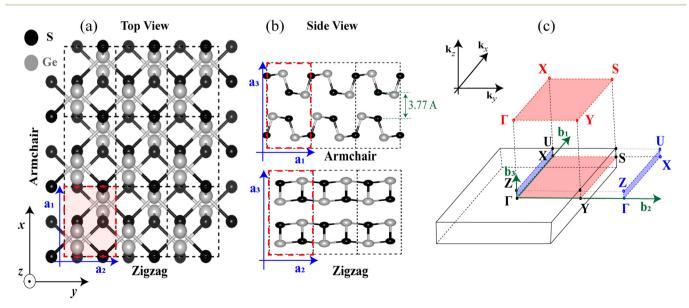
Fig. 2 Illustration of the atomic structure of bulk GeS. (a) Top view of the atomic structure of bulk GeS in a 3 x 3 x 1 supercell. (b) Side views of bulk GeS along the AC and ZZ directions, respectively. (c) The bulk first BZ of an orthorhombic Bravais lattice and its projected surfaces. The gray and black spheres stand for the Ge and S atoms, respectively. The unit cell is indicated by the dashed red rectangle in (a and b).
