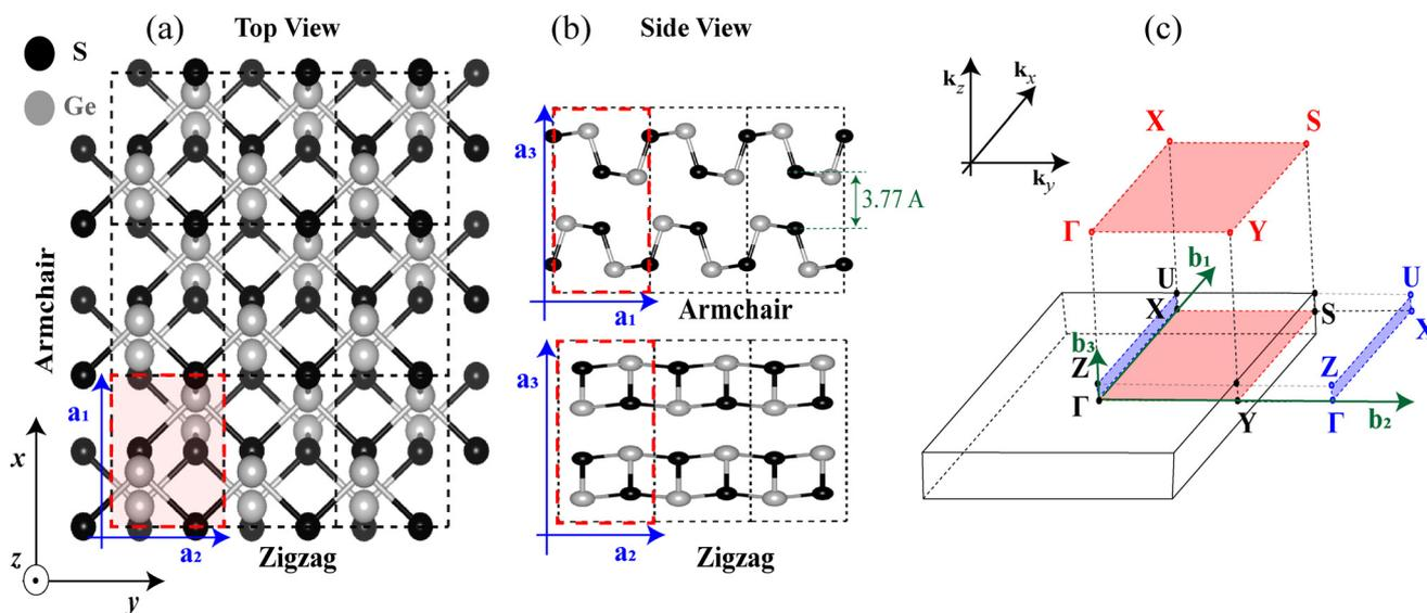
**Fig. 2** Illustration of the atomic structure of bulk GeS. (a) Top view of the atomic structure of bulk GeS in a  $3 \times 3 \times 1$  supercell. (b) Side views of bulk GeS along the AC and ZZ directions, respectively. (c) The bulk first BZ of an orthorhombic Bravais lattice and its projected surfaces. The gray and black spheres stand for the Ge and S atoms, respectively. The unit cell is indicated by the dashed red rectangle in (a and b).
