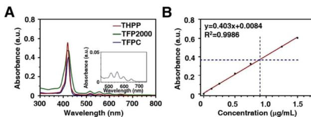
**Fig. 1** (A) UV-vis spectra of free THPP ( $1.0\ \mu\text{g mL}^{-1}$ ), TFP2000 ( $200.0\ \mu\text{g mL}^{-1}$ ), and TFPC ( $50.0\ \mu\text{g mL}^{-1}$ ) in ethanol solution. (B) Normalized absorbance of THPP ethanol solution at varying concentrations (detected at 419 nm). The dashed lines mean the THPP porphyrin portion concentrations calculated from the standard curve with the detected UV absorption values of TFPC ethanol solution.
