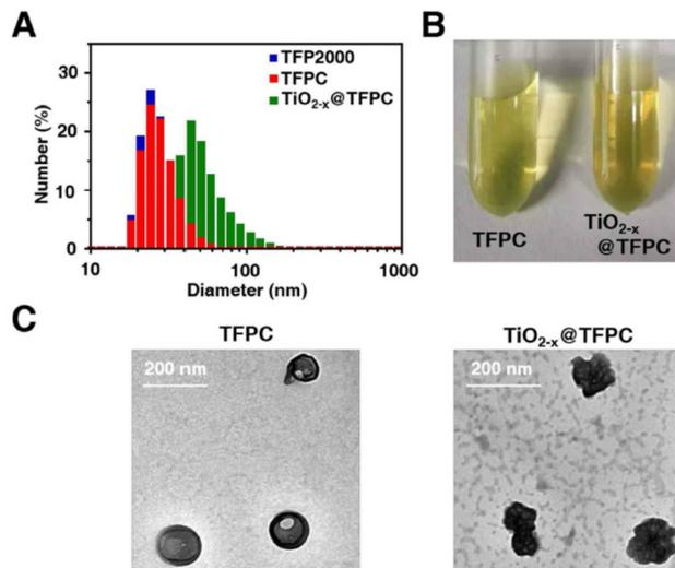
**Fig. 4** Chemophysical characterization of the TFPC nanoparticles and  $\text{TiO}_{2-x}@\text{TFPC}$  nanocomposites. (A) Hydrodynamic diameter. (B) Digital images of TFPC nanoparticles ( $0.4 \text{ mg mL}^{-1}$ ) and  $\text{TiO}_{2-x}@\text{TFPC}$  nanocomposites ( $3 \text{ mg mL}^{-1}$ ) aqueous solution. (C) TEM.
