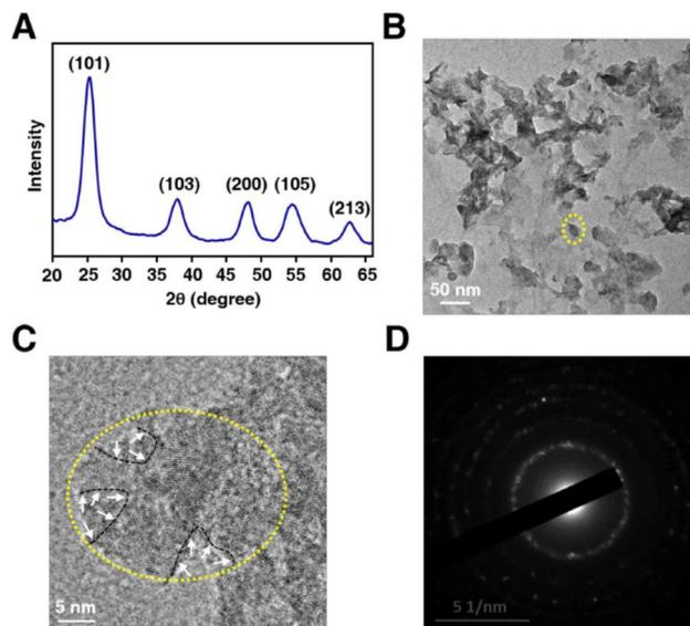
**Fig. 3** (A) XRD patterns, (B) TEM, (C) HRTEM images, and (D) SAED pattern of "black" anatase  $\text{TiO}_{2-x}$ . In (C), black short-dashed curves are applied to outline portions of the interface between the crystalline core and the disordered outer layer (marked by white arrows).
