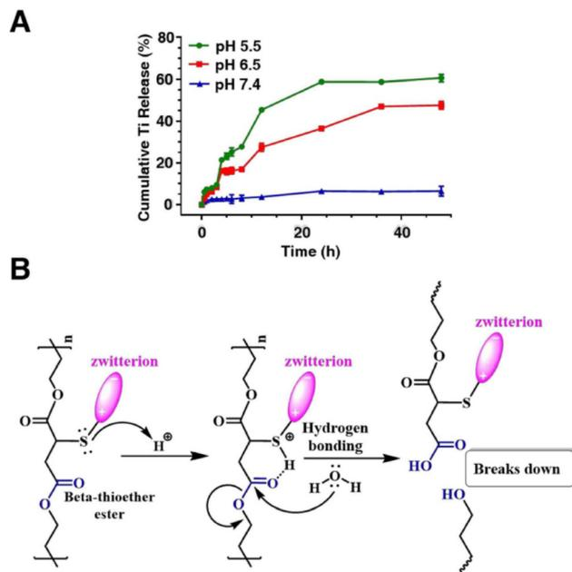
**Fig. 5** (A) The drug release profiles of TiO<sub>2</sub> (expressed as a percentage of Ti release) in the TiO<sub>2-x</sub>@TFPC nanocomposites in aqueous solutions at pH 7.4, pH 6.5, and pH 5.5. (B) The pH-responsive mechanism of the main chains on the polyester containing the beta-thioether ester structure in acidic media.
