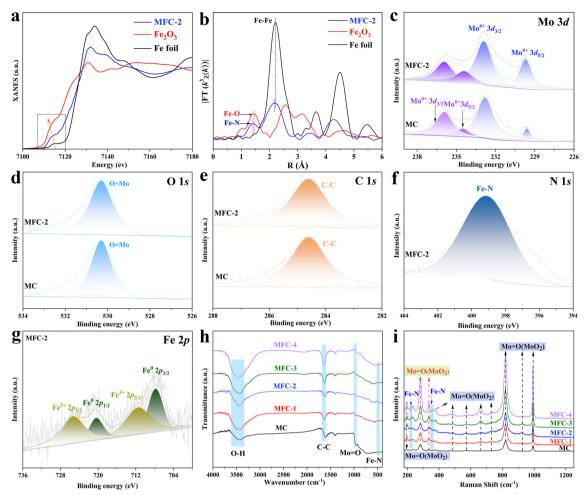
Fig. 2 Characterization of the compositions and chemical states of the as-obtained samples. (a) Normalized Fe K-edge XANES spectra of MFC-2 in reference to Fe foil and Fe<sub>2</sub>O<sub>3</sub>; (b) k<sub>3</sub>-weighted Fourier-transform Fe K-edge EXAFS spectra; (c-g) XPS spectra of MC and MFC-2; (h) FT-IR spectra; (i) Raman spectra.
