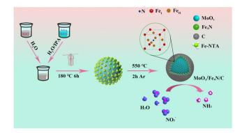
Scheme 1 A tandem disproportionation reaction (Mo<sup>5+</sup>  $\rightarrow$  Mo<sup>4+</sup> + Mo<sup>6+</sup>) and nitridation-carbonation route (Fe<sub>4</sub>N/C) for building a multilayer core-shell MFC catalyst.
