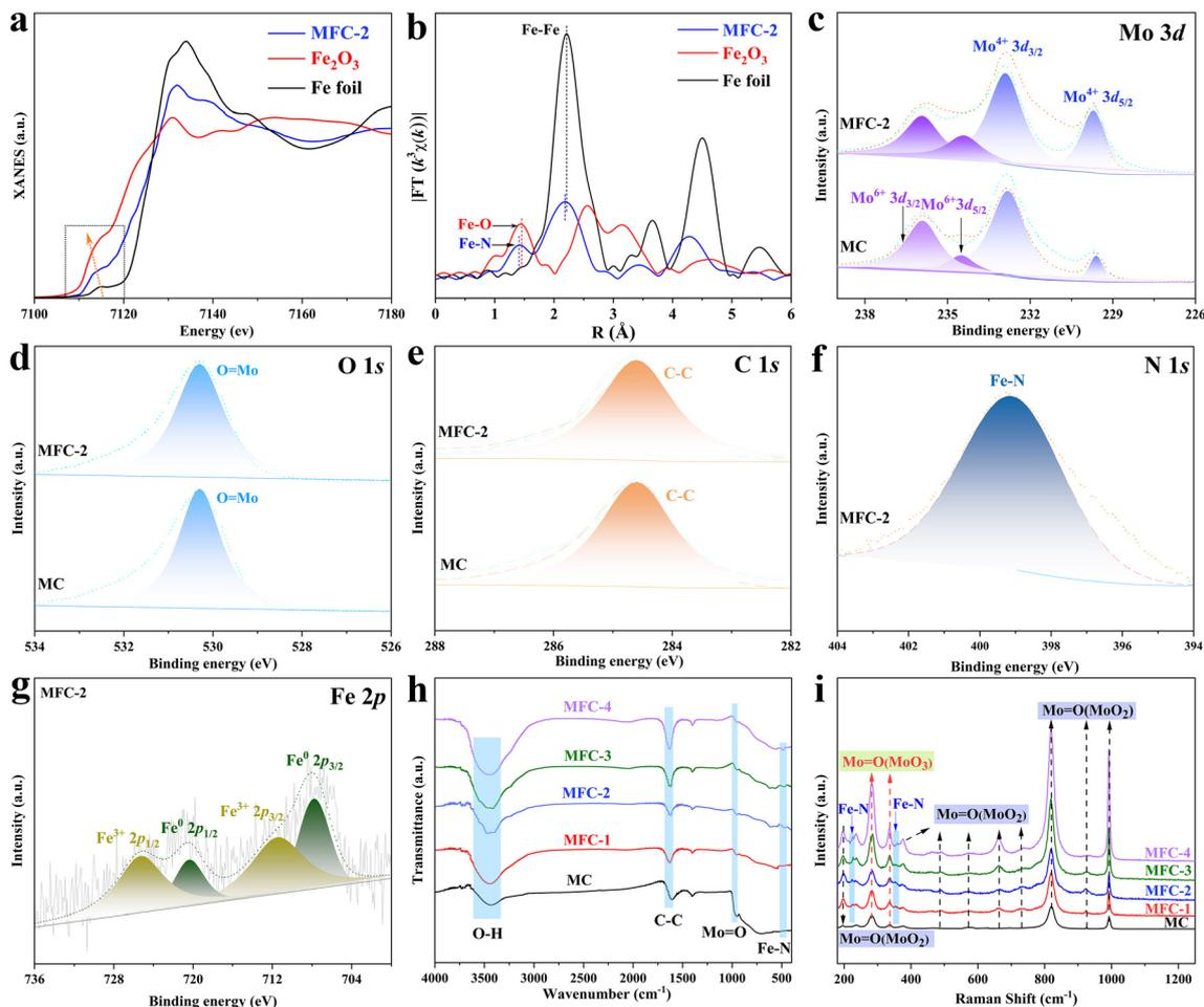
**Fig. 2** Characterization of the compositions and chemical states of the as-obtained samples. (a) Normalized Fe K-edge XANES spectra of MFC-2 in reference to Fe foil and Fe<sub>2</sub>O<sub>3</sub>; (b)  $k_3$ -weighted Fourier-transform Fe K-edge EXAFS spectra; (c–g) XPS spectra of MC and MFC-2; (h) FT-IR spectra; (i) Raman spectra.
