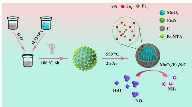
**Scheme 1** A tandem disproportionation reaction ( $\text{Mo}^{5+} \rightarrow \text{Mo}^{4+} + \text{Mo}^{6+}$ ) and nitridation–carbonation route ( $\text{Fe}_4\text{N}/\text{C}$ ) for building a multi-layer core–shell MFC catalyst.
