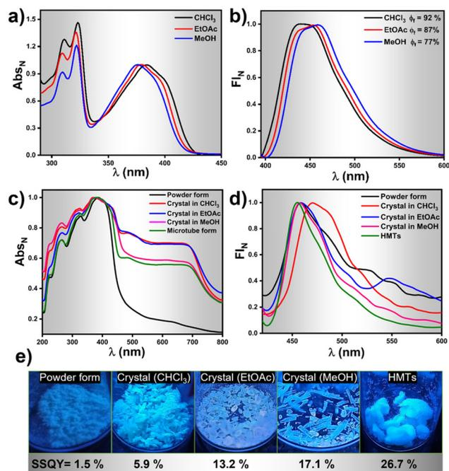
**Fig. 5** Photophysical properties of HNBI-B in solution and solid state. (a and b) Emission and absorption spectra of HNBI-B in CHCl<sub>3</sub>, EtOAc and MeOH ( $\lambda_{\text{ex}}$ -390 nm, 5  $\mu\text{M}$  conc.). (c and d) Solid state absorption and emission spectra of HNBI-B in different forms viz. As-prepared powder form, crystals obtained from CHCl<sub>3</sub>, EtOAc, MeOH and HMTs form. (e) Solid state quantum yield of HNBI-B in each form and photographs taken under UV light.
