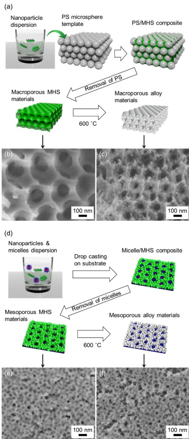
**Fig. 6** Schematic illustration of (a) macroporous and (d) mesoporous alloy materials. SEM images of (b) and (c) macroporous and (e) and (f) mesoporous structures composed of (b) and (e) Co–Ni MHS and (c) and (f) Co–Ni alloy, respectively.
