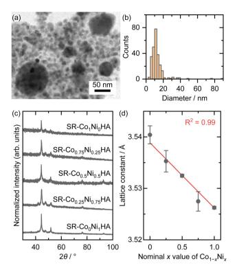
Fig. 5 (a) TEM images and (b) the corresponding particle diameter distribution of SR-Co<sub>0.5</sub>Ni<sub>0.5</sub>HA. (c) XRD patterns and (d) the corresponding lattice constants of SR-Co<sub>1-x</sub>Ni<sub>x</sub>HA (x = 0, 0.25, 0.5, 0.75, 1).
