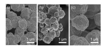
Fig. 3 SEM images of (a) P-Co<sub>1</sub>Ni<sub>0</sub>HA, (b) P-Co<sub>0</sub>Ni<sub>1</sub>HA, and (c) P-Co<sub>0.5</sub>Ni<sub>0.5</sub>HA.
