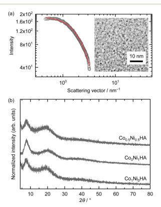
Fig. 2 (a) SAXS pattern of reacting solution of Co<sub>0.5</sub>Ni<sub>0.5x</sub>HA; raw data (black circle) and fitted data (red line). Inset is TEM image of dried Co<sub>0.5</sub>N<sub>0.5x</sub>HA. (b) XRD patterns of dried powders of Co<sub>1</sub>Ni<sub>0</sub>HA, Co<sub>0</sub>Ni<sub>1</sub>HA, and Co<sub>0.5</sub>Ni<sub>0.5</sub>HA.
