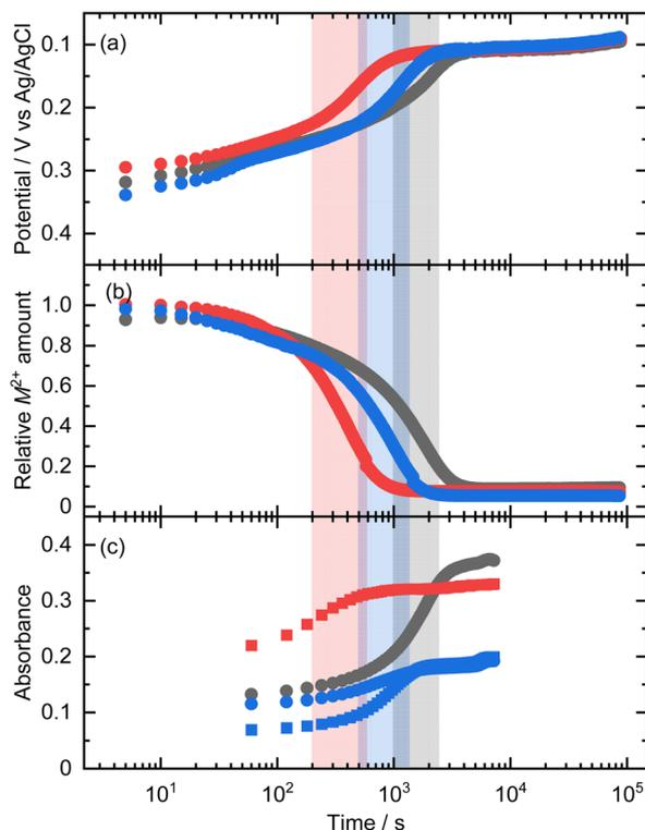
Fig. 1 Time-dependent change of (a) potential, (b) relative ion amounts, and (c) absorbance at 480 nm (circle, Co species) and 400 nm (square, Ni species) of reacting solutions of Co $_2$ Ni $_{10}$ HA (black), Co $_0$ Ni $_1$ HA (red), and Co $_{0.5}$ Ni $_{0.5}$ HA (blue).
