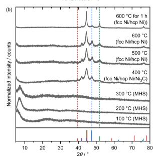
Fig. 4 (a) TG-DTA curves (upper panel) and MS spectra (lower panel) of  $Co_0Ni_1HA$ . (b) XRD patterns of  $Co_0Ni_1HA$  after heat-treatment at 100-600 °C without holding the temperature. The red, blue, and green bars in (b) are  $Ni_3C$  (JCPDS #06-0697), interstitial-atom-free hcp  $Ni^{50}$  (analogous structure of hcp Co #89-7373), and fcc Ni (#04-0850).
