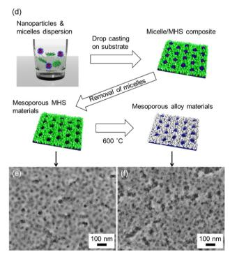
Fig. 6 Schematic illustration of (a) macroporous and (d) mesoporous alloy materials. SEM images of (b) and (c) macroporous and (e) and (f) mesoporous structures composed of (b) and (e) Co-Ni MHS and (c) and (f) Co-Ni alloy, respectively.
