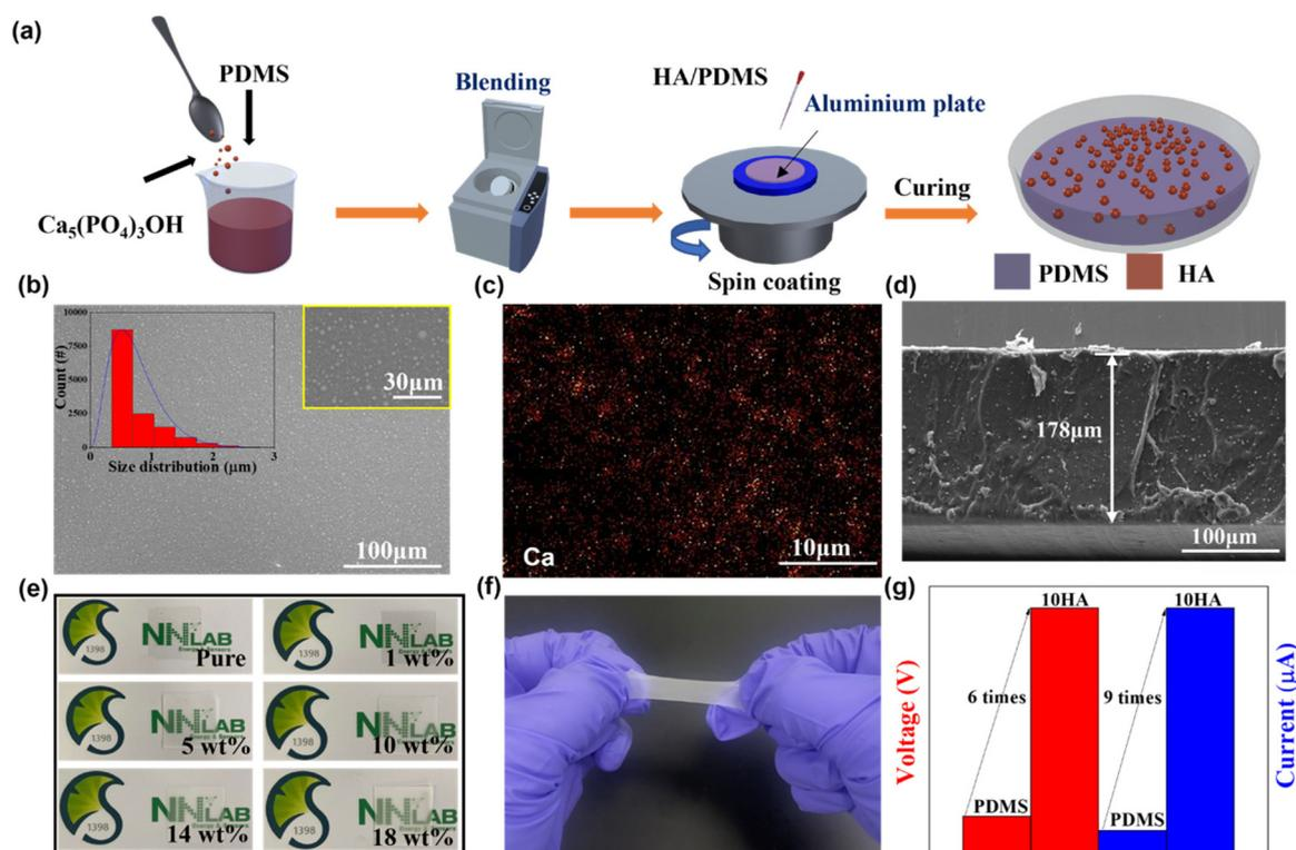
**Fig. 1** (a) Schematic illustration of the fabrication process of HA/PDMS bionanocomposite. (b) 3D structure of HA/PDMS bionanocomposite. (c) FE-SEM images of the HA/PDMS. (d) Energy dispersive spectrometry (EDS) images of the HA/PDMS bionanocomposite. (e) Cross-sectional FE-SEM image of the bionanocomposite. (f) Photographs demonstrating the stretchability of HA/PDMS. (g) Enhancing output performance of triboelectric nanogenerator via HA/PDMS compared to pristine PDMS.
