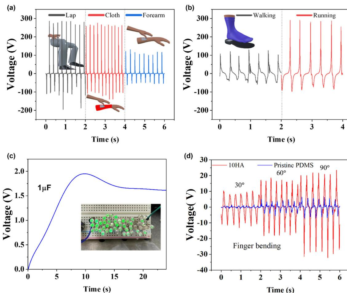
**Fig. 6** HA-TENG as a skin-patchable encodable touch sensor and wearable sensor for human activities. (a) Various HA-TENG applications attached on various substrates (e.g., lap, cloth, forearm) and their triboelectric output voltages. (b) Schematic of HA-TENG-implanted insole and its triboelectric output voltages. (c) LED lighting and capacitor charging are possible after 10 min of running. (d) Comparison of voltage response caused by finger bending between pristine PDMS and 10HA/PDMS.
