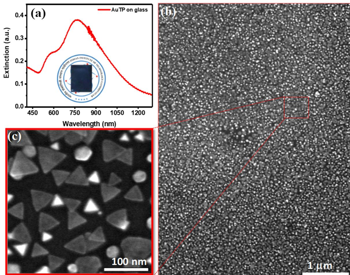
**Fig. 1** (a) UV-visible extinction spectra of AuTP attached to the glass substrate. The inset shows the photo of the AuTP functionalized glass substrate. (b) Corresponding SEM image of the AuTP functionalized on ITO substrate. The scale bar is 1  $\mu\text{m}$ . (c) The zoom-out SEM image of AuTP. The scale bar is 100 nm.
