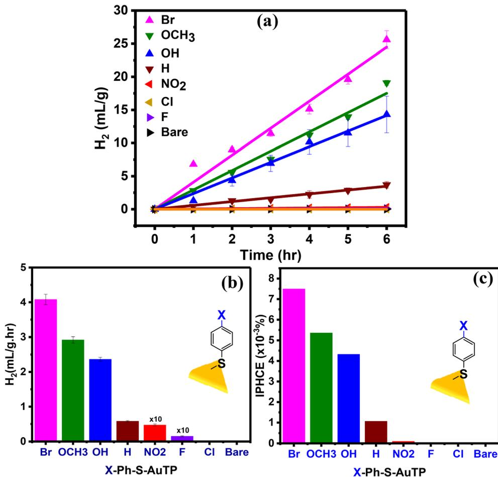
Fig. 3 (a) Photocatalytic H<sub>2</sub> production observed over time for various X-Ph-S-AuTP substrates, (b) the H<sub>2</sub> production rate, and (c) IPHCE calculated for each substrate. The experiment was performed in neutral water under 808 nm laser illumination with a power density of 100 mW cm<sup>-2</sup>.
