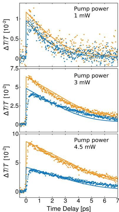
**Fig. 5** Measured and simulated transient signals at the polariton resonances of the gold–TDBC core–shell nanorods pumped with 1 mW, 3 mW and 4.5 mW (from top to bottom). The dots mark the experimental results while the solid lines represent the simulations. The signal along the upper polariton is indicated by the blue marks, and the signal along the lower polariton is indicated by the orange marks.
