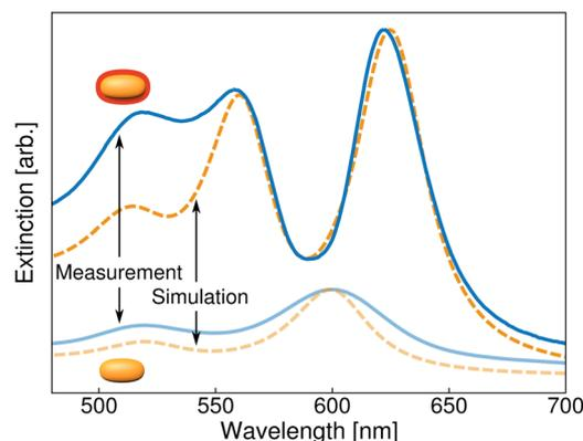
**Fig. 3** Measured and simulated static extinction spectra of bare and TDBC-coated gold nanorods. The solid blue lines represent the experimental data, and the dashed orange lines represent the simulations. The two lower lines describe the bare particles whereas the two upper lines describe the coupled situation.
