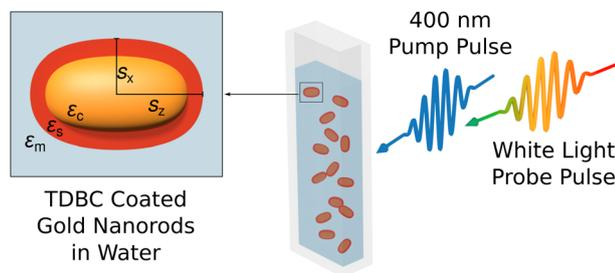
**Fig. 1** Sketch of the experimental setting: TDBC coated gold nanorods were dissolved in water and excited using a 400 nm pump pulse. A white light probe pulse detected the change in transmission after the excitation. A magnified particle is shown on the left with the parameters used later in the simulations.
