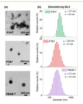
Fig. 2 (a) TEM images of P3HT, PTB7 and PBDB-T NPs with 9:1 polymer: Pluronic® relative mass concentration. (b) Size distribution obtained by DLS:  $\mu$  and  $\sigma$  correspond to the mean and the standard deviation, respectively.
