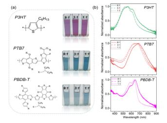
Fig. 1 (a) Chemical structures of the commercial conjugated polymers used in this work and photographs of the corresponding polymeric colloids obtained, at three polymer: Pluronic® F127 relative concentrations. (b) UV-vis absorption spectra of NP aqueous dispersions.
