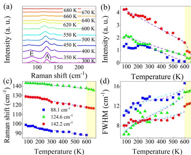
**Fig. 4** (a) Raman spectra of GeTe at different temperatures. Temperature dependence of the peak intensity (b), position (c), and FWHM (d) of the three Raman modes, where the dashed lines represent the fit results or act as a guide for the eyes.
