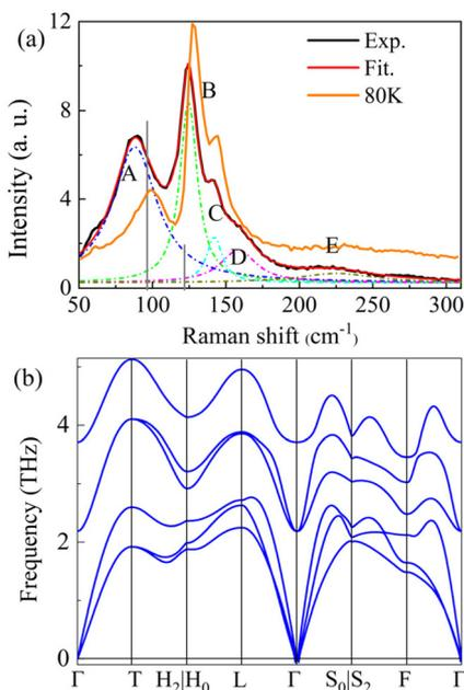
**Fig. 2** (a) Raman spectrum of bulk GeTe at room temperature; solid curve – experimental result (red); vertical lines – calculated values (black). (b) The calculated phonon dispersion relations of bulk GeTe.
