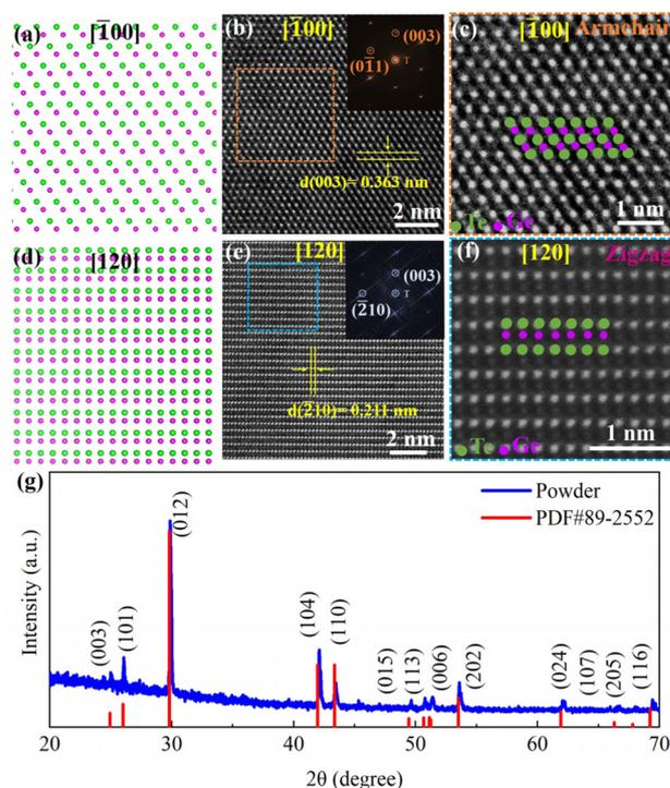
**Fig. 1** (a) and (d) Simulated structure of  $\alpha$ -GeTe along  $[\bar{1}00]_R$  and  $[120]_R$  zone axes. (b) and (e) The HAADF-STEM images of  $\alpha$ -GeTe taken along  $[\bar{1}00]_R$  and  $[120]_R$  zone axes; the insets show the corresponding fast Fourier transform (FFT) patterns. (c) and (f) Zoomed-in images of the square regions in (b) and (e), respectively, for the corresponding AC and ZZ directions. (g) The powder XRD pattern of  $\alpha$ -GeTe at room temperature.
